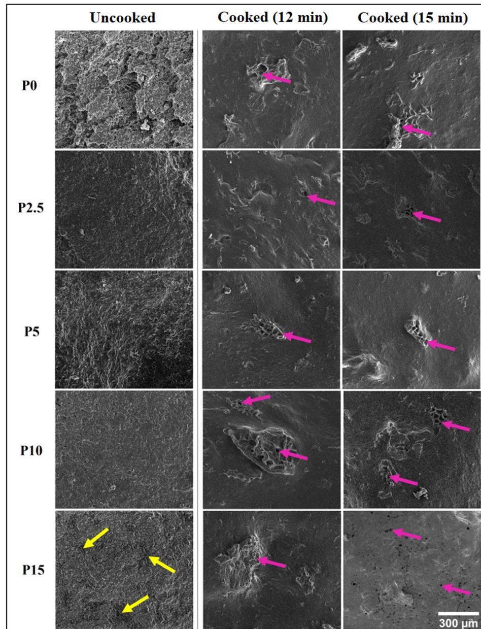
**Figure 5.** FESEM micrographs of all the pasta samples (yellow arrows indicate defects on the surface of the pasta, whereas pink arrows indicate pores). (Magnification: 250 $\times$ ).
