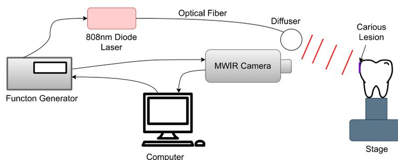
**Figure 1.** Block schematic of the thermophotonic imaging system: the bacteria-induced caries is highlighted by the purple rectangle and is positioned normal to the MWIR camera.
