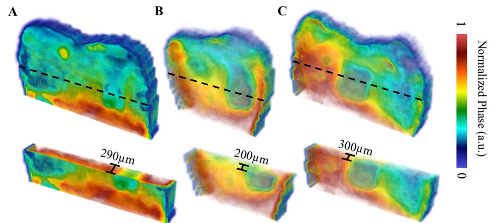
**Figure 7.** TC-PCT LIOP reconstructions with partial transparency of the (A) buccal, (B) distal, and (C) lingual surfaces using a 0.2–0.6 Hz, 12 s chirp with 40 ms pulse width and 20 ms slice width. All reconstructions were filtered using the histogram equalization filter [13] to improve the caries visibility. The dashed black lines indicate the regions of the cross-sectional cuts (displayed underneath the whole volume). Volumes are displayed using software available online [31].
