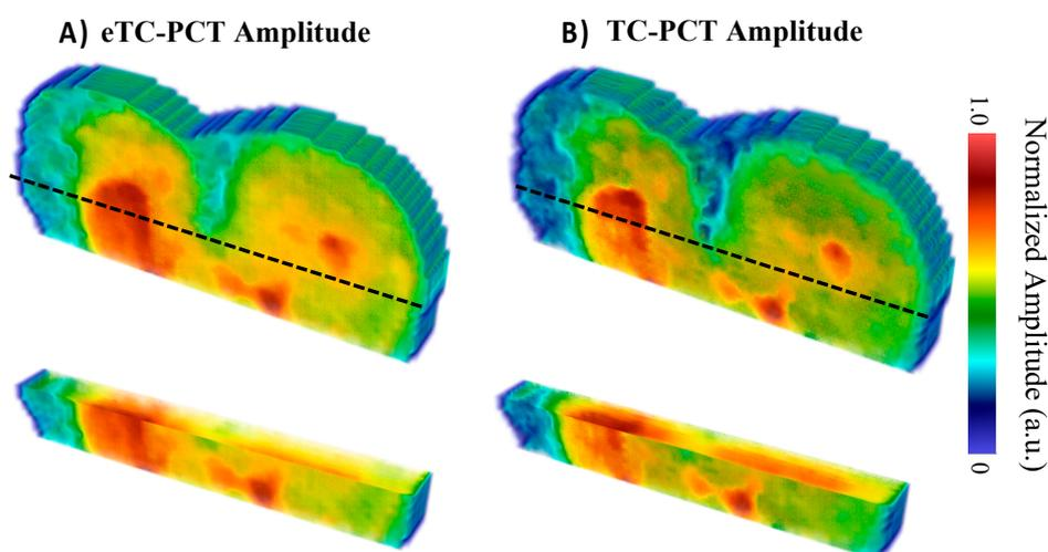
**Figure 13.** Amplitude reconstructions of the M8 sample (8 days of cariogenic biofilm exposure) using the (A) eTC-PCT and (B) TC-PCT algorithms with 20 ms slice widths. The amplitudes were normalized between 1.0 and 0 by subtracting the minimum amplitude value and then dividing by the maximum amplitude value within each slice. Volumes are displayed using the method of [31].
