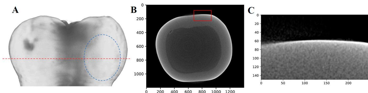
**Figure 12.**  $\mu$ -CT results of sample M8 (8 days of demineralization): (A) Volume reconstruction with no visible lesion. The dashed blue oval indicates the region where the lesion is visible with the naked eye, the dashed red line indicates the plane where the transverse view B is taken. (B) Transverse view of the sample with the red box indicating where the lesion should be visible. (C) Enlarged view of the red box seen in B, with no lesion visible.
