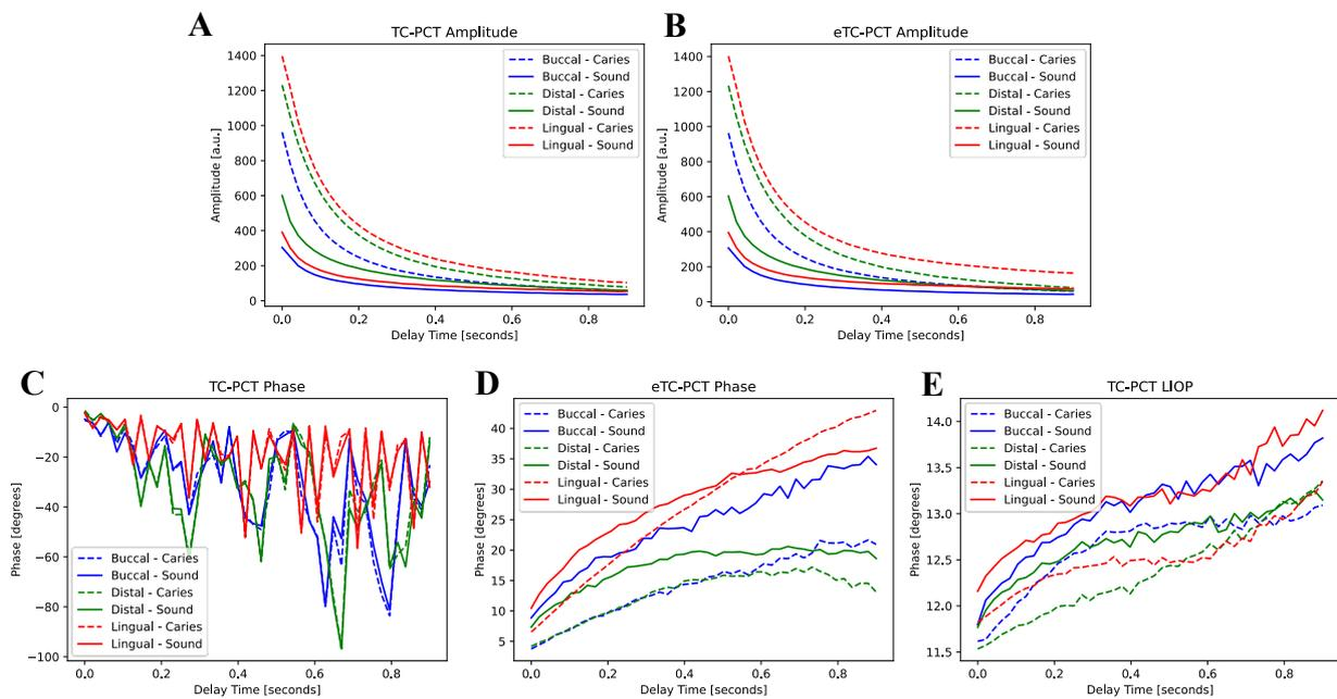
**Figure 5.** Mean amplitude and phase responses of the caries lesions and sound enamel regions highlighted in Figure 4 for (A) TC-PCT amplitude, (B) eTC-PCT amplitude, (C) TC-PCT phase, (D) eTC-PCT phase, and (E) TC-PCT LIOP.
