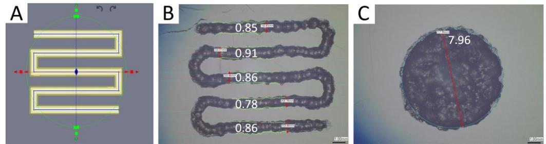
**Figure 2.** GelMA/OMA printability. A three-line print was designed in TSIM (A) which produced the lines shown (B) and the disc (C) using the settings in Table 1. All measurements are in mm. Scale bar 1mm.
