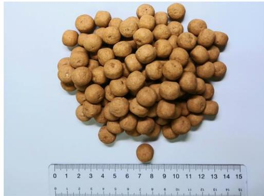
**Figure 5.** The loess bio-balls manufactured by the LW method. The diameter of the loess bio-ball is about 1.3 mm.
