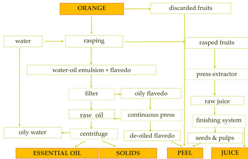
Figure 2. Main processing steps of orange processing industry.
