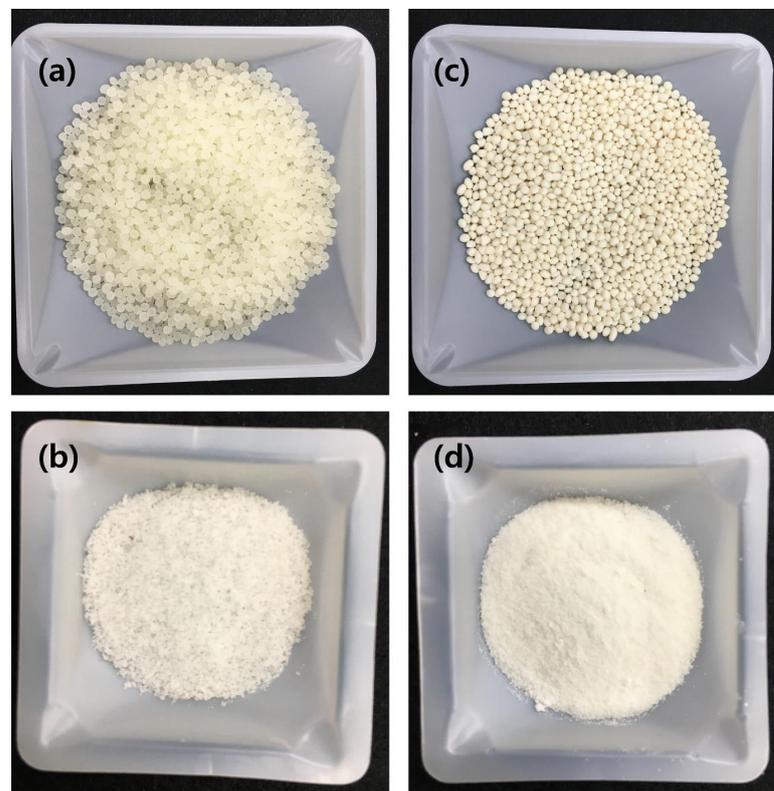
**Figure 1.** The images of raw and ground bioplastics (particle size  $\leq 0.5$  mm) ((a) raw PLA resin particle, (b) ground PLA, (c) raw PHA resin particle, (d) ground PHA).
