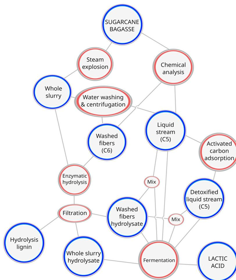
**Figure 1.** Experimental setup for lactic acid production from sugarcane bagasse.
