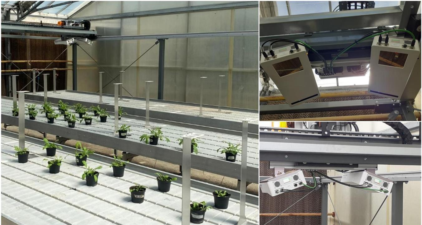
**Figure 1.** The Phenospex phenotyping platform of CREA—Research Centre for Vegetable and Ornamental Crops (Pontecagnano, Italy). On the left, the overview of the pot experiment is shown; vertical bars carry the coordinates (barcodes), allowing the 3D scanner to recognize the position of plants on the bench. On the right, details (front–bottom) of the PlantEye F500 dual scanner are shown.
