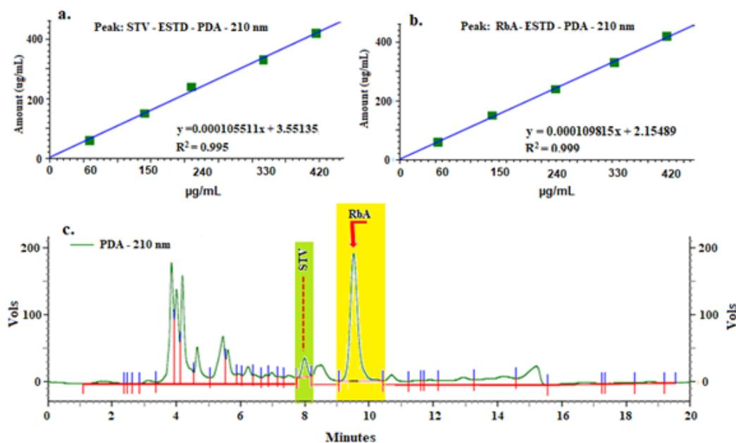
**Figure 2.** Chromatographic analysis of the samples in HPLC, reading of the data provided by the software and their analysis and processing. Stevioside calibration curve (a): Rebaudioside A calibration curve (b), and Chromatogram of analyzed leaf sample (c).
