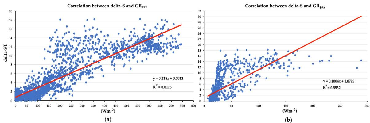
**Figure 5.** Graph of surface temperature difference between unvegetated and vegetated façades ( $\Delta ST$ ) and incident global solar radiation (GR). (a)  $\Delta ST$  correlation with GR detected on the external plant canopy of the green cover ( $GR_{ext}$ ); (b)  $\Delta ST$  correlation with GR detected inside the gap ( $GR_{gap}$ ), which was the 60 cm space between the building’s vegetated façade and the green cover shading it.
