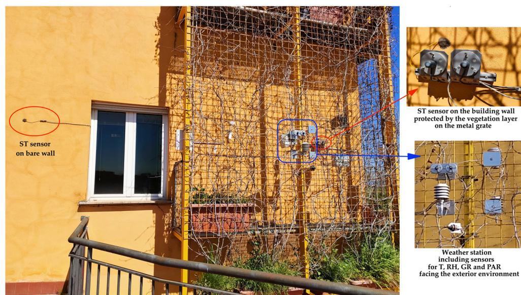
**Figure 2.** Section of the building at ENEA Casaccia RC showing the steel infrastructure sustaining vegetation in the SW façade at the first-floor level. The picture was taken in March, when the deciduous *Parthenocissus quinquefolia* (L.) Planch. Was still bare after losing its leaves in winter. On the
