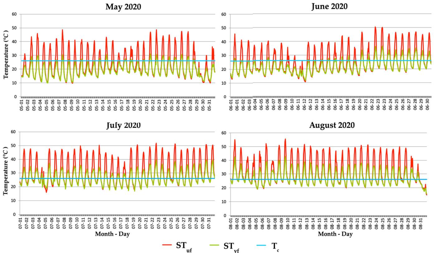
**Figure 4.** Surface temperature (°C) registered on the vegetated façade shaded by *Parthenocissus* ( $ST_{vf}$ , green line) and on the unvegetated façade ( $ST_{uf}$ , red line). The light blue horizontal line at 26 °C indicates the value of the indoor comfort temperature inside the building ( $T_c$ ).
