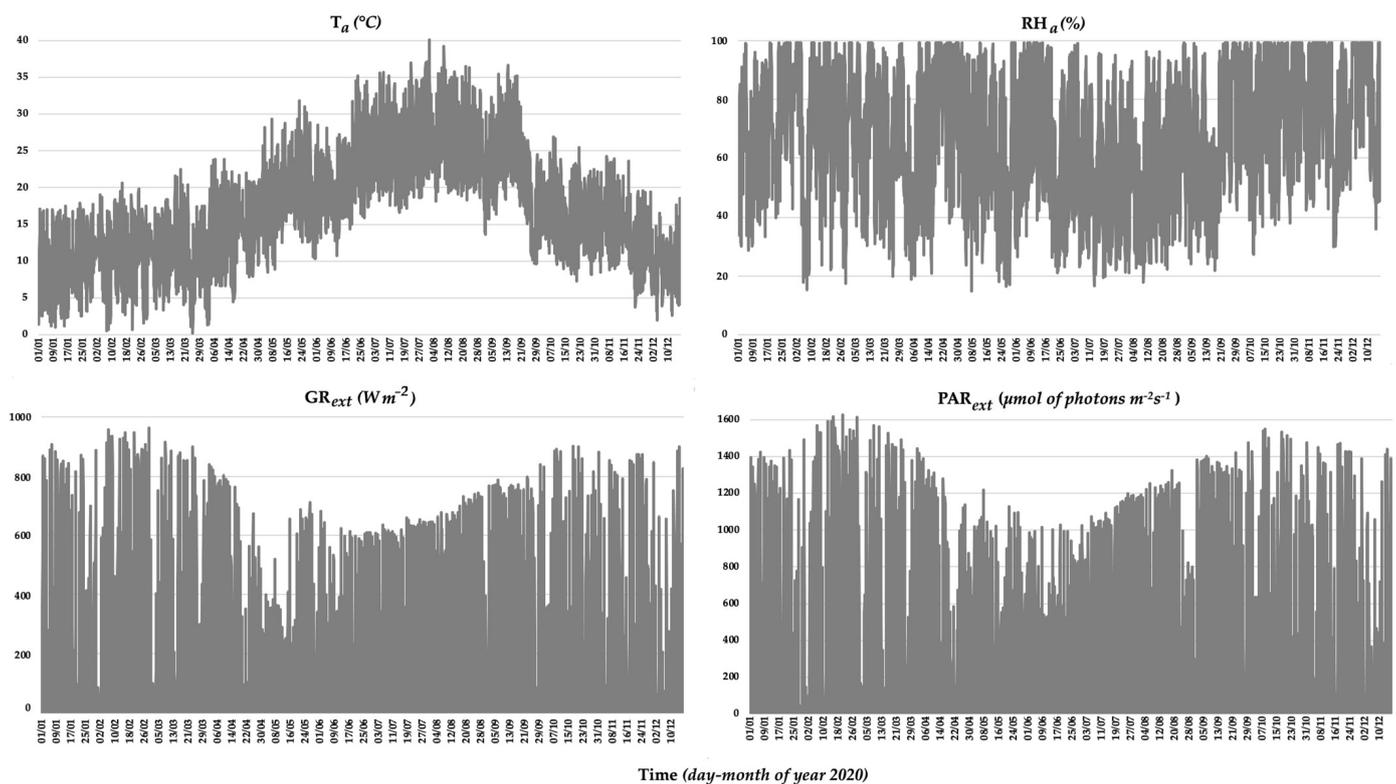
**Figure 3.** Hourly data recorded in 2020 of the ambient temperature and relative humidity measured on the external side of the vegetated façade ( $T_a$  and  $RH_a$ , respectively) in the upper part of the figure, and of the solar global radiation and photosynthetically active radiation measured parallel to the vegetated façade on the external side ( $GR_{ext}$  and  $PAR_{ext}$ , respectively) in the lower part of the figure. On the x-axis, the time is expressed as day–month of 2020.
