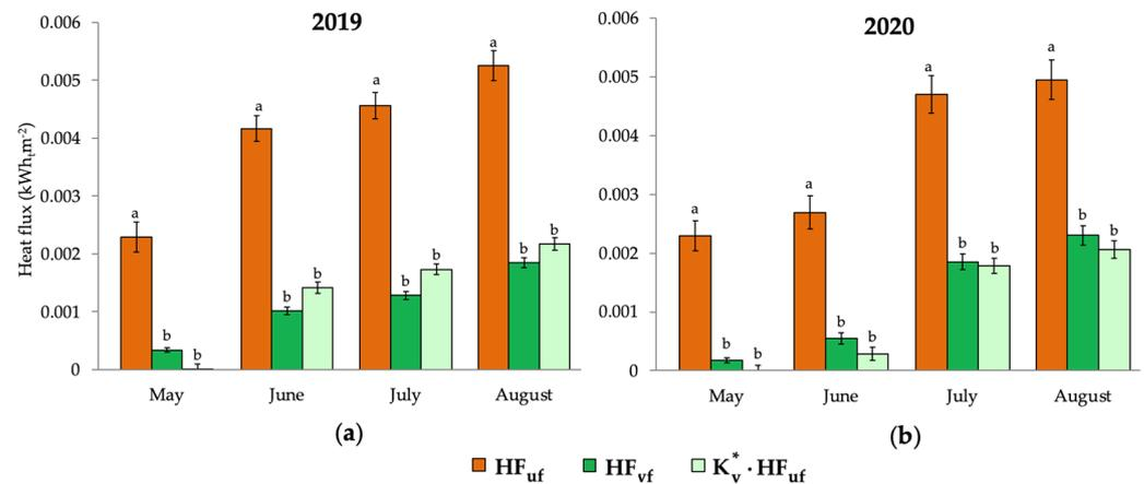
**Figure 9.** Mean value of hourly heat fluxes entering the interior of the building calculated from May to August 2019 (a) and 2020 (b). Unvegetated façade HF ( $HF_{uf}$ , in orange), vegetated façade HF ( $HF_{vf}$ , in green) and  $K_v^* HF_{uf}$  (in light green). Error bars show  $\pm$  SEM (standard error of the mean), different letters indicate statistically significant differences ( $p < 0.01$ ).
