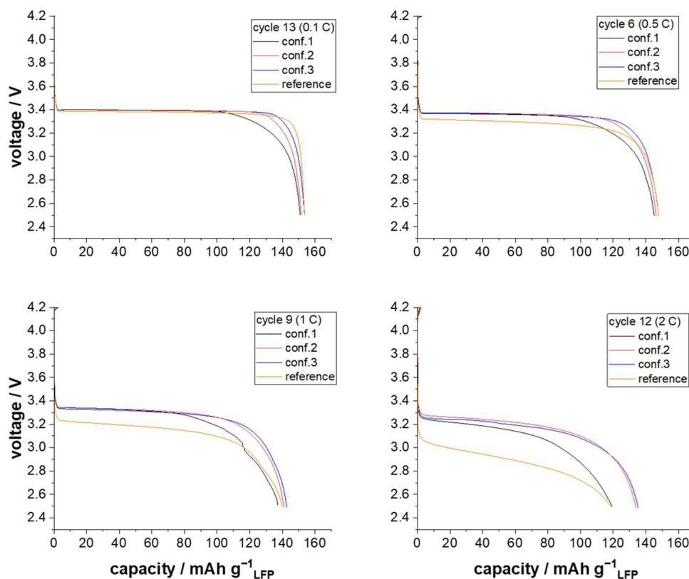
**Figure 6.** Voltage over capacity plots for the discharge rate of 0.1 (cycle 13), 0.5 (cycle 6), 1 (cycle 9), and 2 C (cycle 12) in dependency of different processing strategies.
