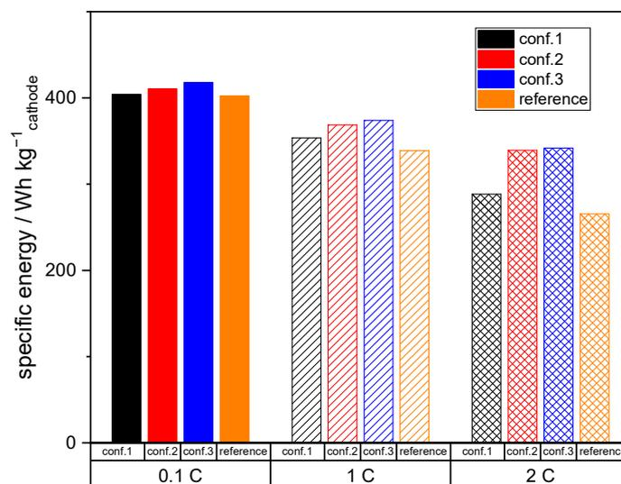
**Figure 7.** Specific energy at the cathode level at 0.1 (cycle 13), 1 (cycle 9), and 2 C (cycle 12) in dependency of different processing strategies.
