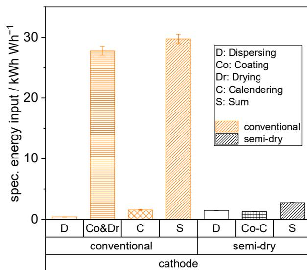
**Figure 8.** Specific energy consumption of electrode manufacturing steps dispersing, coating, drying, and calendaring for the conventional and semi-dry process route at the same throughput.
