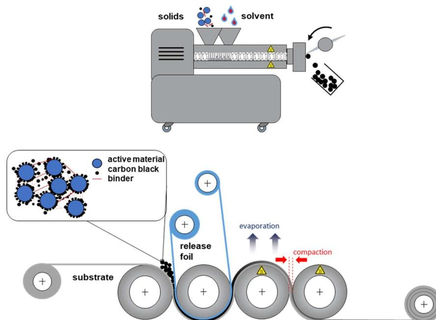
**Figure 1.** Schematic drawing of LFP cathode production using twin-screw extrusion for dispersing and a calender for coating.
