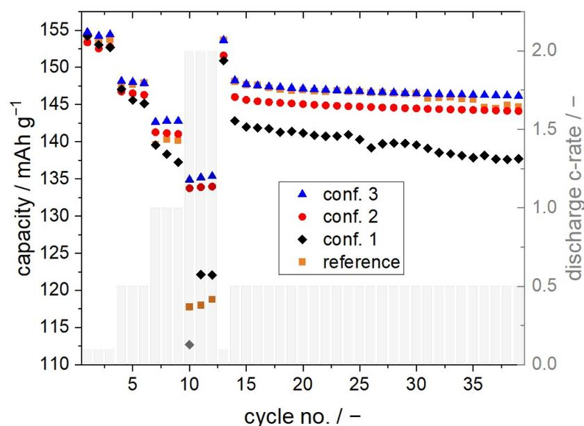
**Figure 5.** Specific discharge capacities for half cells in dependency of different manufacturing strategies.
