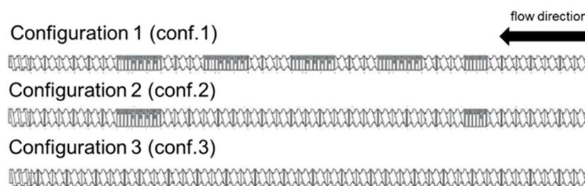
**Figure 2.** Types of screw configurations used with varying kneading and conveying elements.
