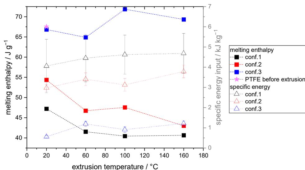
**Figure 3.** Melting enthalpy and specific energy input in dependency of extrusion screw configuration and temperature.
