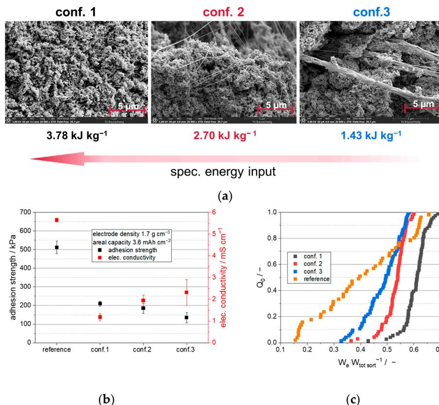
**Figure 4.** (a) SEM pictures of cathode granules in dependency of different screw configurations; (b) adhesion strength and electric conductivity in dependency of different dispersion strategies; (c) sum distribution of relative elastic work in dependency of different manufacturing strategies measured by nanoindentation.
