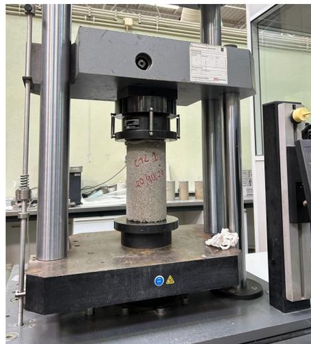
**Figure 7.** Compressive strength test on a concrete specimen.
