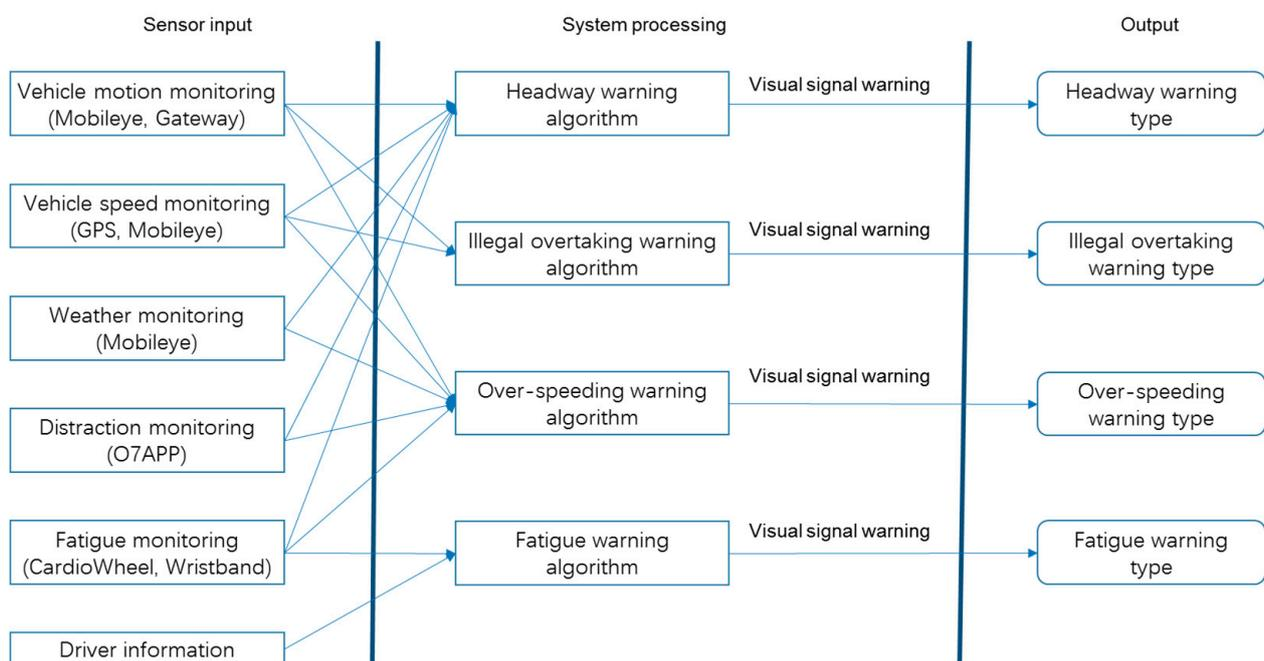
**Figure 1.** The architecture flow diagram for the integrated ADAS (own illustration).
