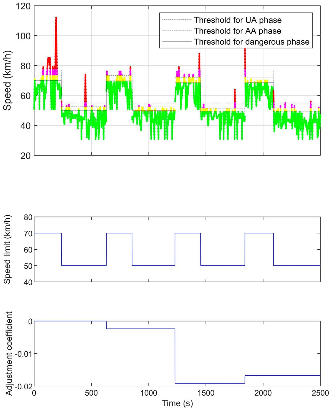
**Figure 8.** A test example of the real-time over-speeding warning algorithm.
