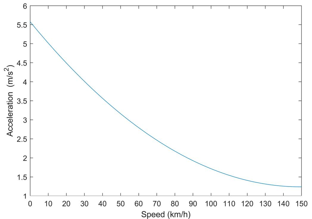
**Figure 4.** The relationship between the safe acceleration and speed (own illustration).
