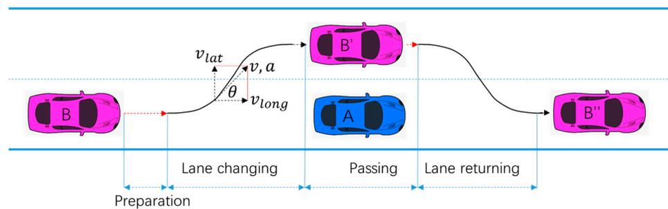
Figure 2. The phases of overtaking move (own illustration).
