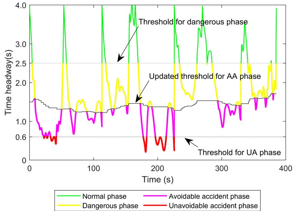
Figure 6. A test example of the adaptive headway warning algorithm ( $a_1 = 0.05, a_2 = 0.06$ ).
