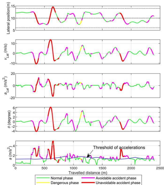
Figure 7. A test example of the real-time illegal overtaking warning algorithm.
