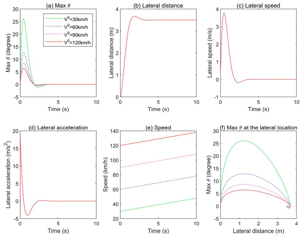
**Figure 3.** The change in max theta, latitudinal variables, and current speeds over time in the lane-changing phases for different initial speeds (for  $a = 0.5 \text{ m/s}^2$ ) (own illustration).
