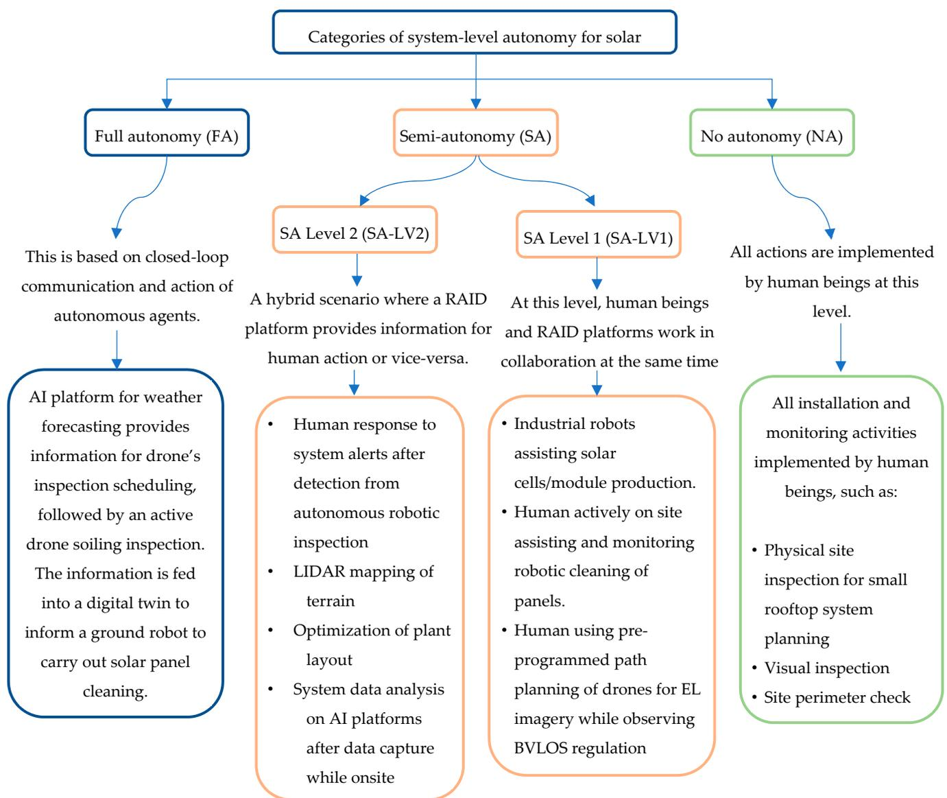
Figure 2. System-level autonomous categories in solar photovoltaics.
