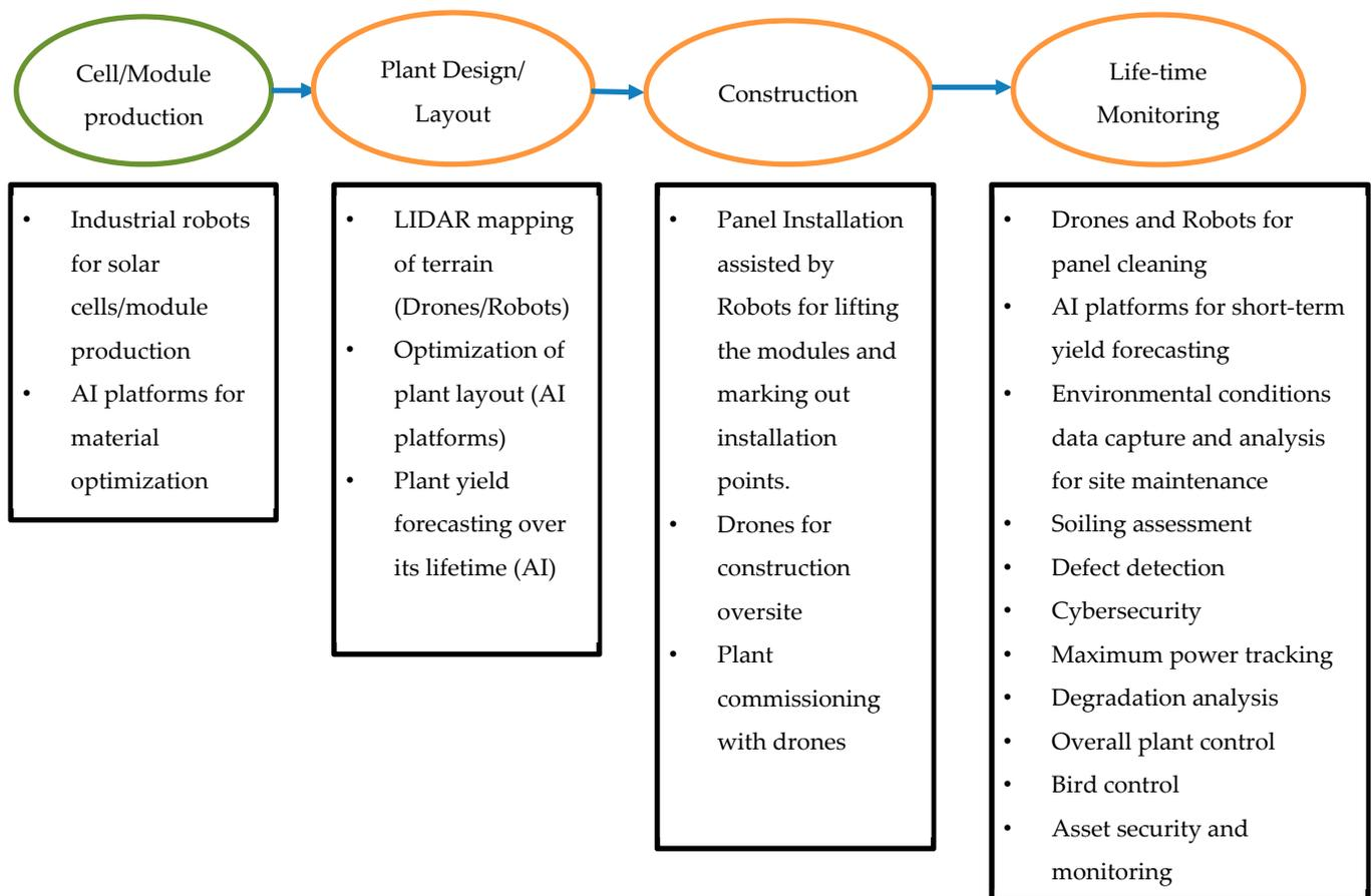
**Figure 1.** Autonomous tasks within Solar PV life cycle.
