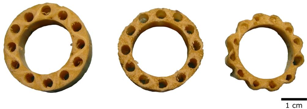
**Figure 16.** “Technical plant stem” in various versions, such as single- or double-braid and circular or star-shaped outline.
