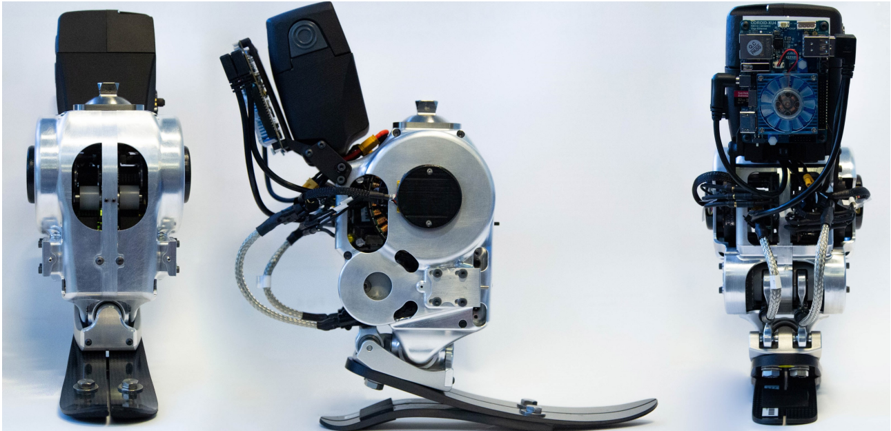
Figure 1. Overview of the 2-DoF ankle prosthesis, which is designed for untethered mobility, tailored for individuals around 75 kg, and suitable for varied terrains.
