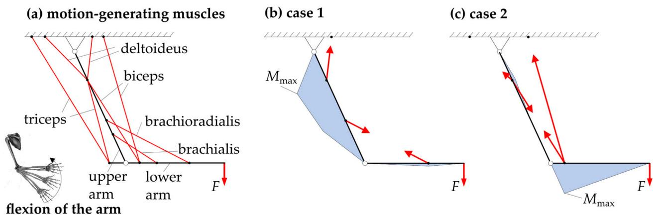
**Figure 1.** Demonstration of the principle of redundancy: the flexion of the human arm by the kinematic overdetermination of the motion-generating muscles according to [13]. The red lines are the labelled muscles and the red arrows are selected associated muscle forces.
