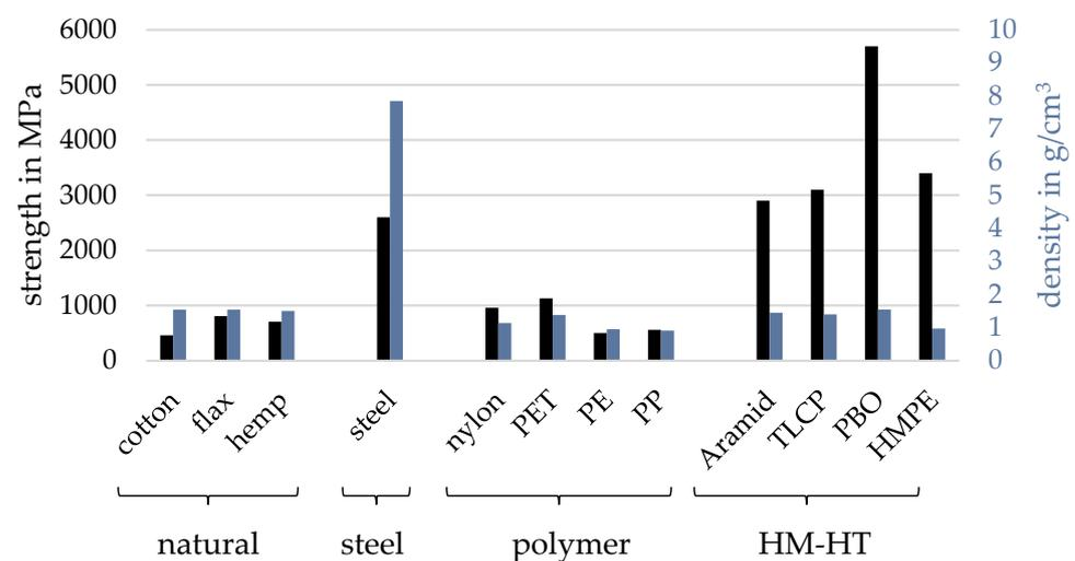
**Figure 3.** Strength and density of major rope fibers, based on [63].
