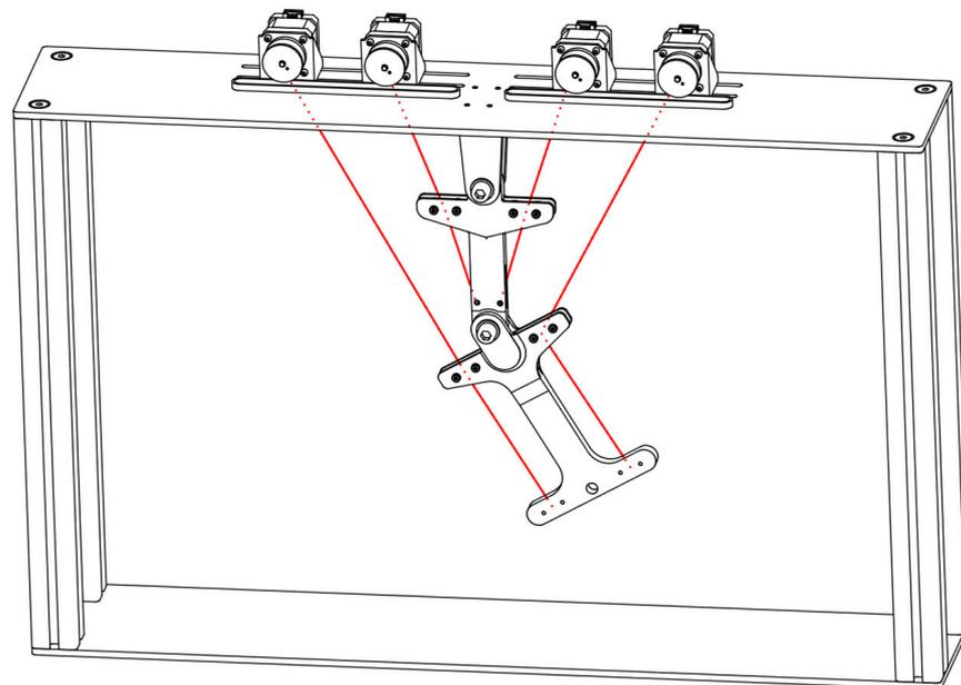
**Figure 7.** Final design of the rope pull demonstrator. The partially concealed rope pulls are shown in red.
