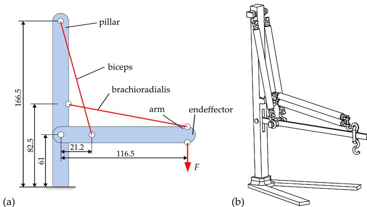
**Figure 5.** Schematic (a) and the final design (b) of the artificial muscle demonstrator.
