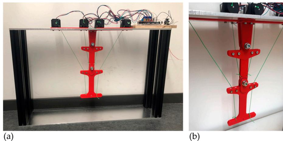
**Figure 8.** Overall view of the manufactured rope pull demonstrator (a) and detailed view of the robot arm (b).
