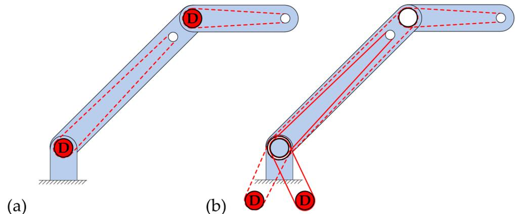
**Figure 4.** Options for the arrangement of the drives (Ds) of the rope pulls for the movement of the arm segment: joint drives (a) and drives mounted outside the moving elements (b). The rope pulls are shown in red. In order to be able to distinguish rope pulls that belong together, some of them are shown as dashed or solid lines.
