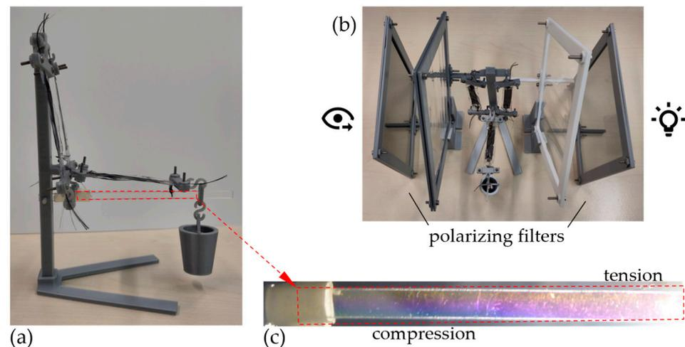
**Figure 6.** Overall view of the manufactured artificial muscle demonstrator (a), the photoelasticity setup (b), and the detailed view of the loaded PC arm (c).
