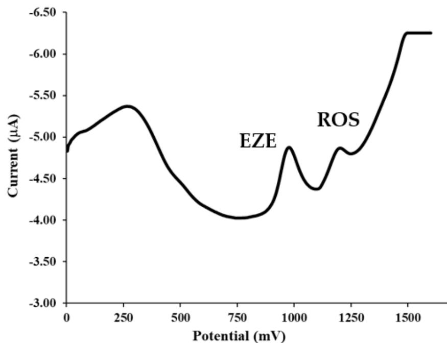
**Figure 1.** The AdSDPV voltammograms of  $5.0 \times 10^{-6}$  M EZE and  $7.5 \times 10^{-6}$  M ROS in 0.1 M  $\text{H}_2\text{SO}_4$  (stripping conditions: accumulation potential of 0.0 V and accumulation time of 15 s).
