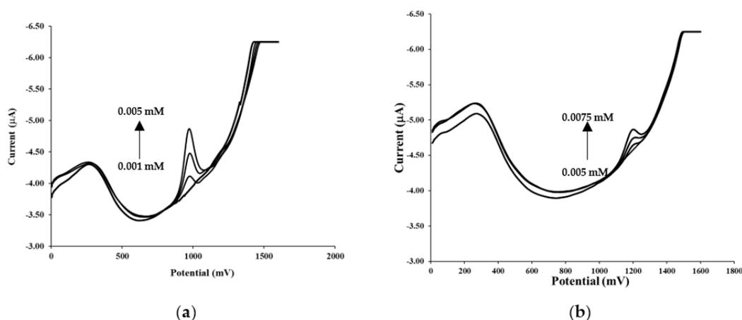
**Figure 5.** AdSDPV of sensor in various concentrations of (a) EZE and (b) ROS using the AdSDPV technique in 0.1 M H<sub>2</sub>SO<sub>4</sub> (stripping conditions: accumulation potential of 0.0 V and accumulation time of 15 s).
