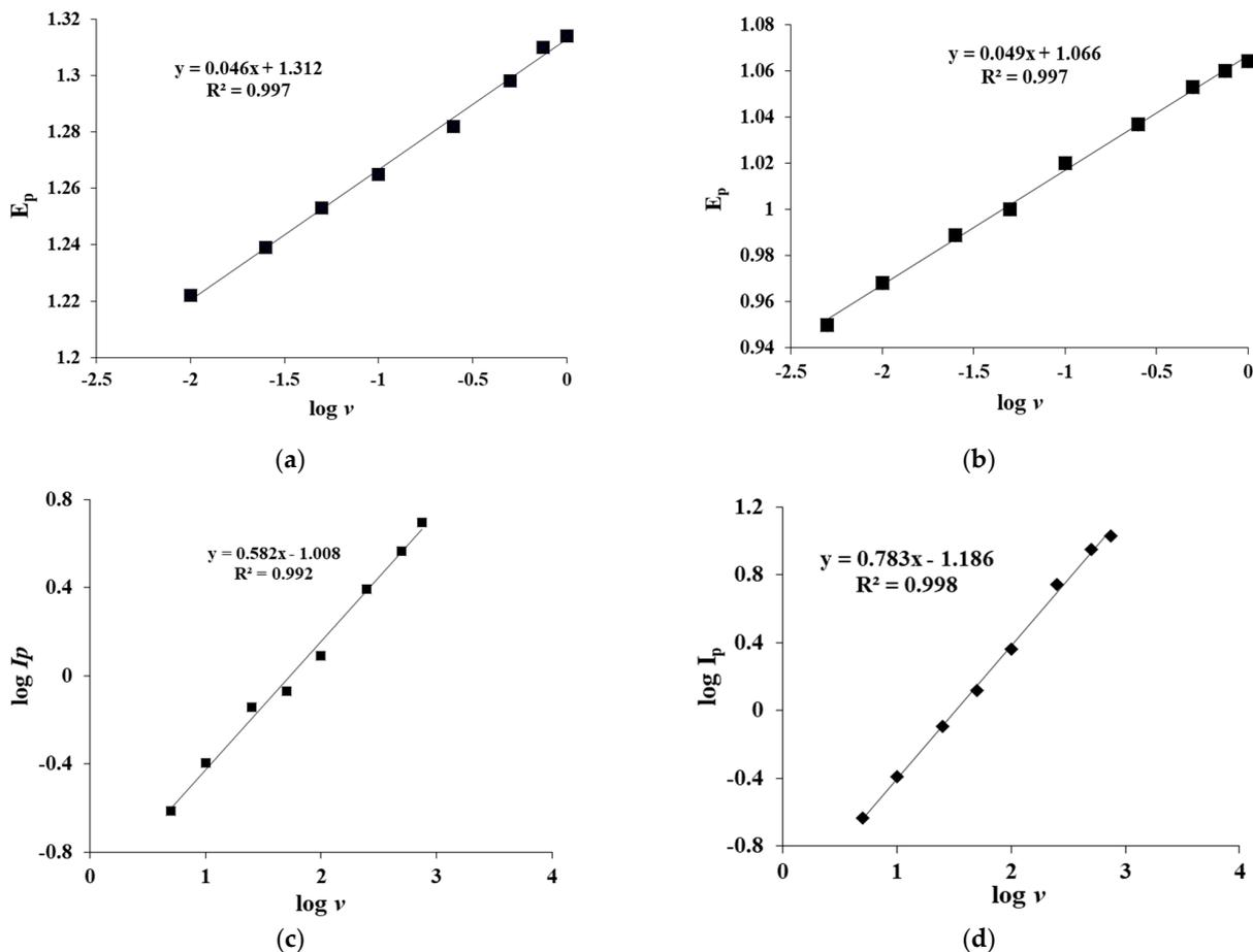
**Figure 3.** Results of scan rate studies: (a)  $E_p$  vs.  $\log v$ , (b)  $\log I_p$  vs.  $\log v$  for 0.1 mM ROS, (c)  $E_p$  vs.  $\log v$ , and (d)  $\log I_p$  vs.  $\log v$  for 0.1 mM EZE in H<sub>2</sub>SO<sub>4</sub>.
