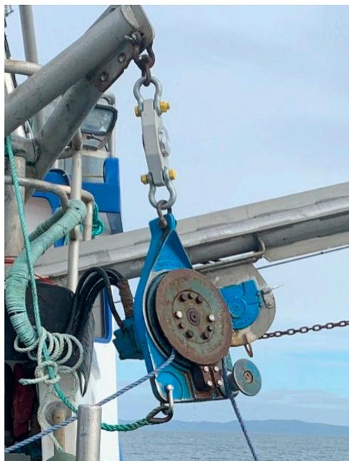
**Figure 4.** Picture of the Euroload load-cell (ELT24) installed above the hauler aboard the FV Island Voyager fishing vessel during the experiment.
