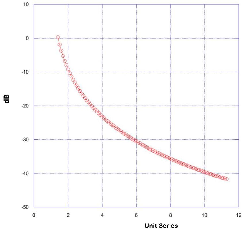
**Figure 8.** The attenuation curve of the optimized isolation system is shown in dB and is a function of the ratio between the mechanical excitation frequency and the resonance frequency of the system which is 1.5 Hz. The curve is theoretical and is taken from an application note present in the Angst + Pfister pneumatic suspension catalog.
