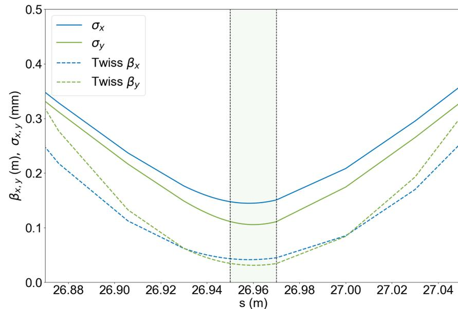
**Figure 7.** OPAL-simulated RMS beam size and beta functions around the waist position. Note that the RMS quantities of all the bunches (projected) are shown. The green shaded area indicates a dielectric tube region 2 cm in length.
