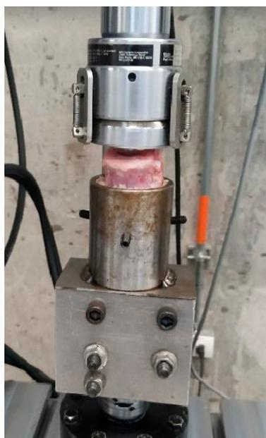
**Figure 2.** Compression test of porcine vertebrae.
