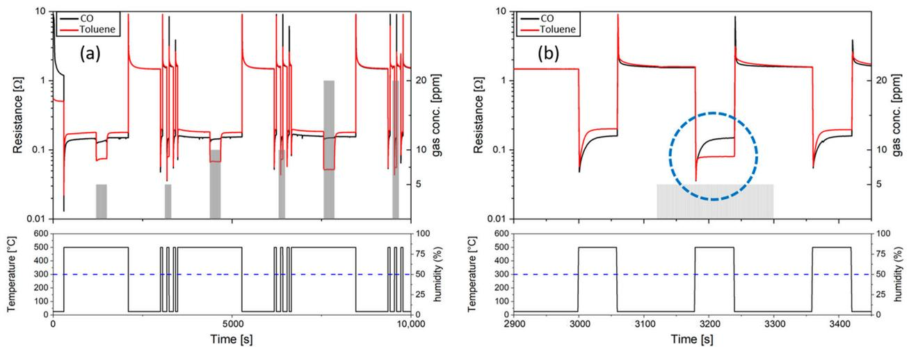
**Figure 1.** (a) Typical resistance measurement in DC- and pulsed-mode T operation for CO and C<sub>7</sub>H<sub>8</sub> (5, 10, and then 20 ppm). (b) Comparison of pulsed-mode T operation for 5 ppm of CO and C<sub>7</sub>H<sub>8</sub>.
