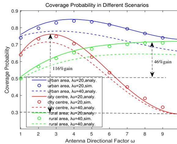
**Figure 2.** Relationship between coverage probability and  $\omega$  under different scenarios. The environment parameters ( $a, b$ ) are set to be (5.3, 0.45), (10.12, 0.16), and (23.2, 0.07) for the rural area, urban area, and city center, respectively.
