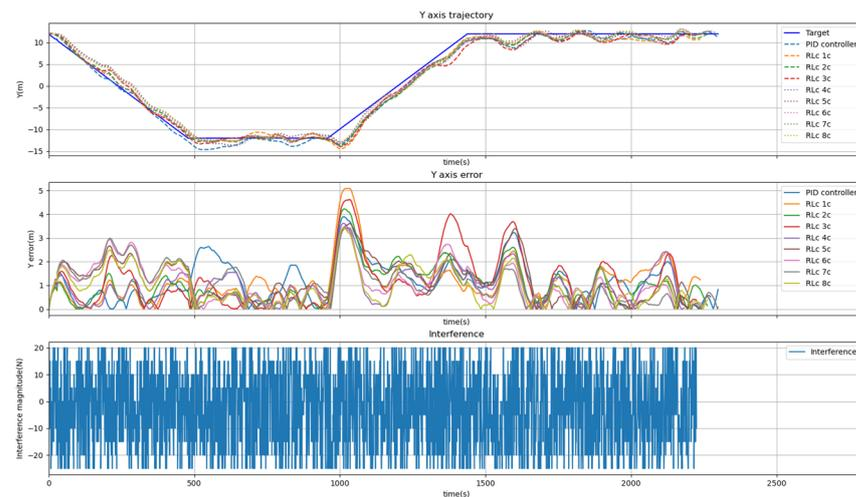
Figure 28. Y-axis dynamic tracking response in the continuous-interference environment.
