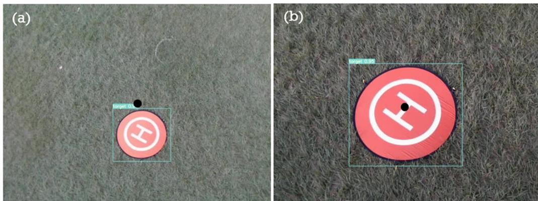
**Figure 6.** Screen obtained during the actual flight. (a) 10 m above the ground (b) 5 m above the ground. The black dot in (a,b) indicates the center of the camera screen while the green box is the Yolo's identified visual screen.
