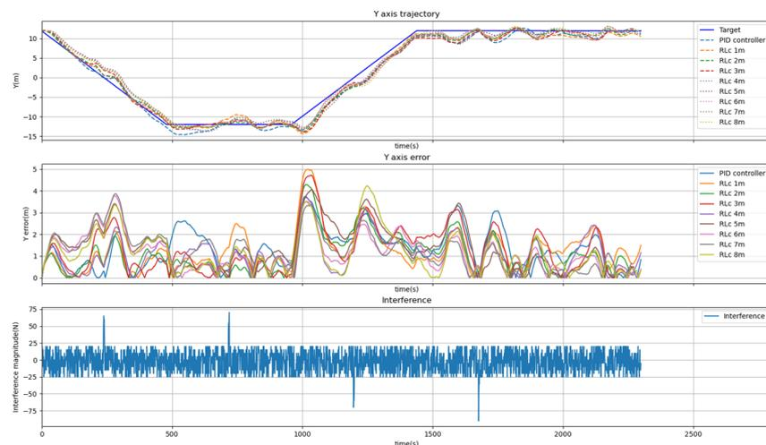
Figure 30. Y-axis dynamic tracking response in the mixed-interference environment.
