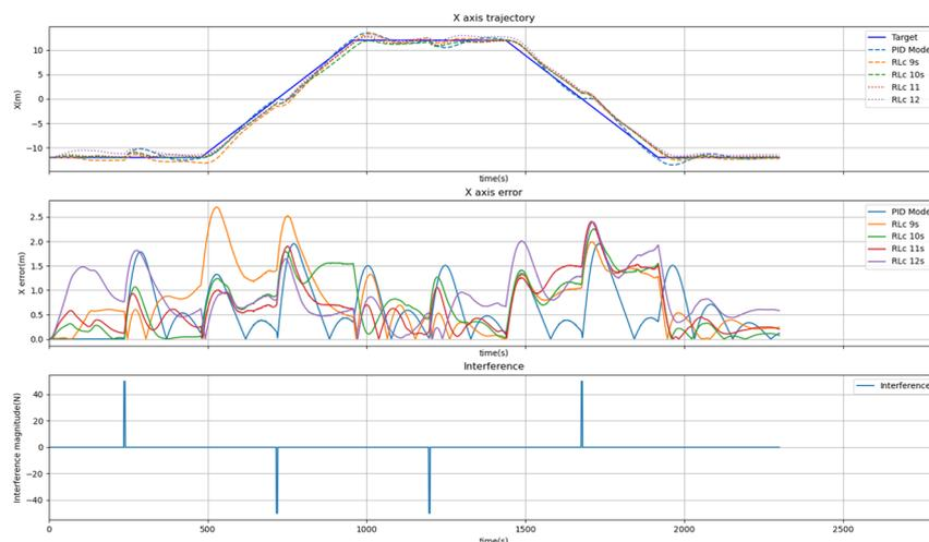
**Figure 32.** X-axis dynamic response in the transfer-learning single-interference environment.
