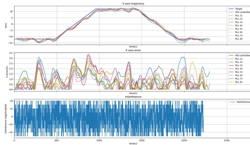
Figure 27. X-axis dynamic tracking response in the continuous-interference environment.
