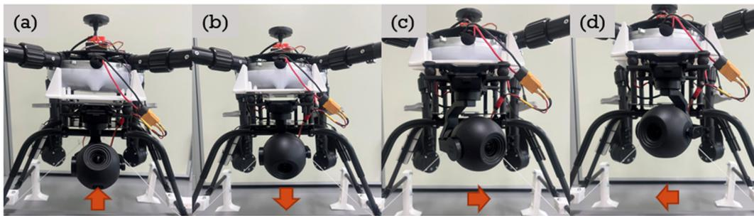
**Figure 9.** The diagram of actual drone's gimble movement (a) up (b) down (c) left (d) right.
