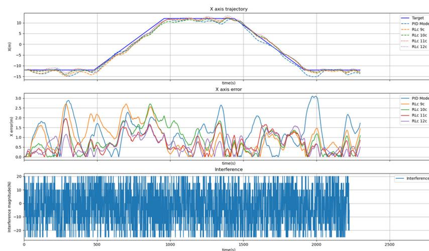
Figure 34. X-axis dynamic response in the transfer-learning continuous-interference environment.
