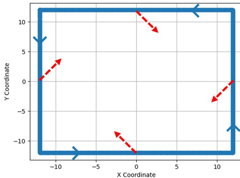
Figure 24. The trajectory (blue) of the target moves along a square of 30 m<sup>2</sup> and with a windy interference (red).
