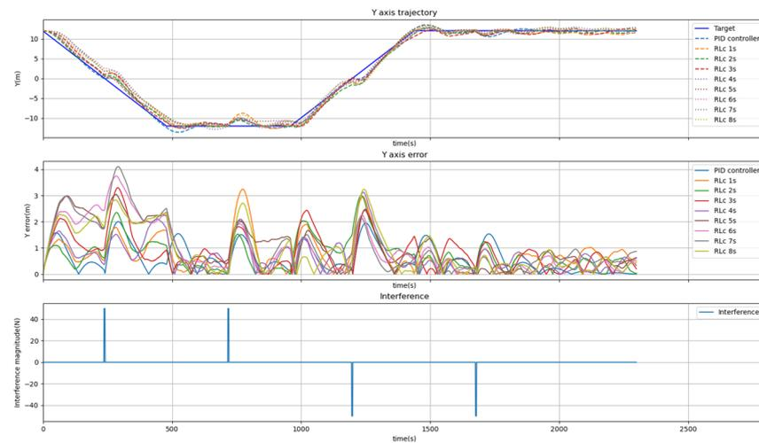
Figure 26. Y-axis dynamic tracking response due to single-interference environment.
