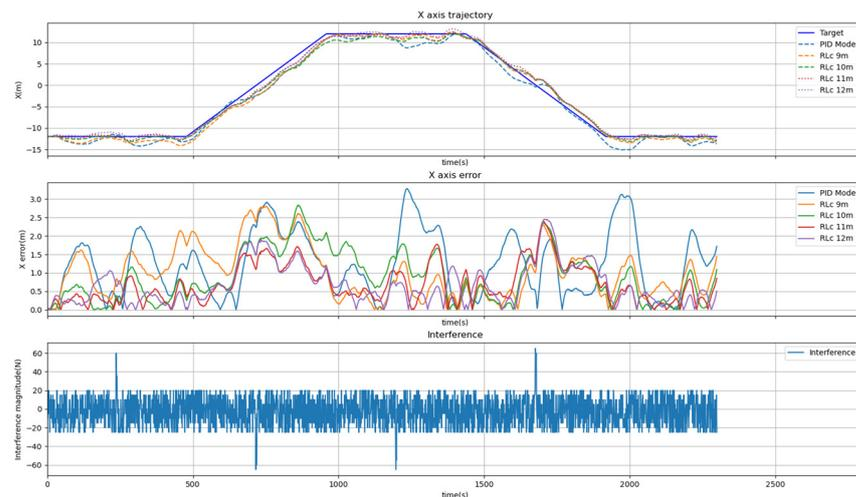
Figure 36. X-axis dynamic response in the transfer-learning mixed-interference environment.
