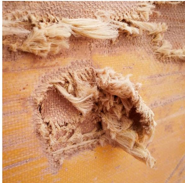
**Figure 1.** Damage to belly guard.
