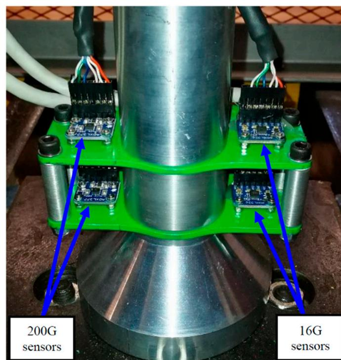
**Figure 11.** Accelerometer mounting.
