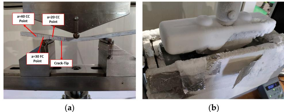
**Figure 4.** ENF test performed in (a) RT environment; (b) LN2 environment.
