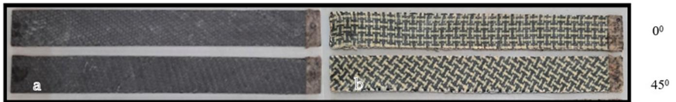
**Figure 5.** Test samples: (a) carbon fibre 0° and 45°, (b) carbon–Kevlar 0° and 45°.
