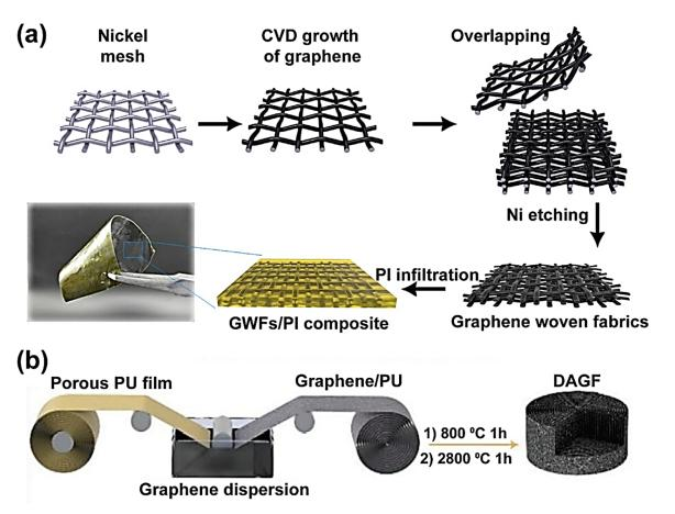
**Figure 4.** (a) Preparation process of GWFs/PI composite films and (b) preparation of dual-assembled graphene framework (DAGF) and composites by rolling process. Reprinted with permission from refs. [57,58].
