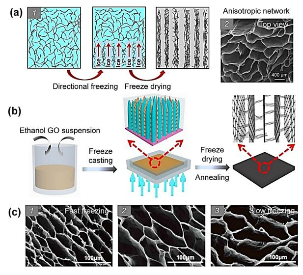
**Figure 5.** (a) Schematic of the microscopic sequences of directional freezing and top view of the final structure [59]. (b) Schematic of directional freezing of graphene oxide (GO) suspension and aligned graphene (GA) structure [60]. (c) SEM images showing vertically aligned graphene networks, fabricated through freeze-drying at different freezing rates, as indicated, and subsequent freeze-drying, captured from a top view [61]. Reproduced with permissions from refs. [59–61].
