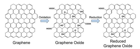
**Figure 2.** Different types of graphene. The chemical structures of graphene, graphene oxide, and reduced graphene oxide, along with their respective synthesis processes. Adopted with permission from ref. [23].
