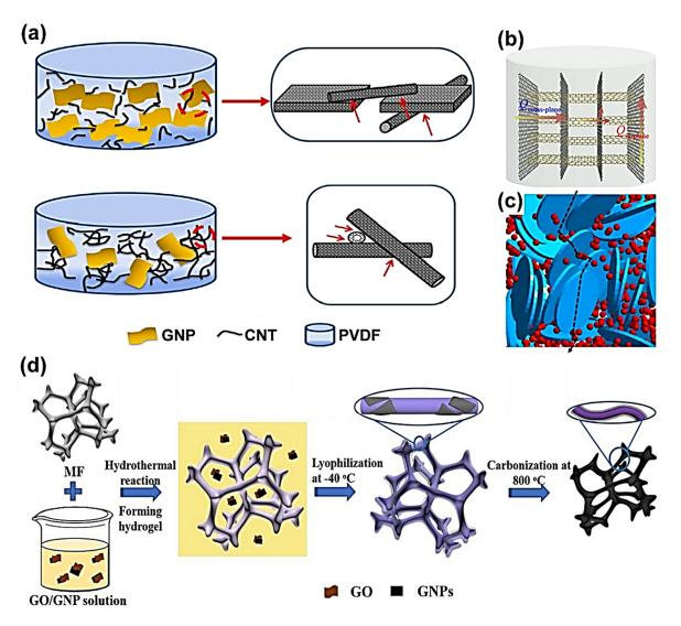
**Figure 7.** (**a**,**b**) Diagrams illustrating the synergies between GNPs and CNTs in thermal conduction [64,65]. (**c**) Schematics illustrating the synergies between GNPs (polymeric nanoalloys, represented by the blue slices) and BN (boron nitrate, represented by the red spheres) [66]. (**d**) Schematic illustration of the preparation process of both the graphene/MF foam (mixed fiber graphene foam) and the derived graphene/carbon foam [67]. Reprinted with permission from refs. [64–67].
