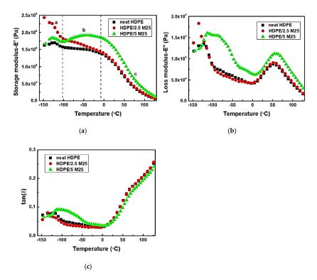
**Figure 3.** The storage modulus (**a**), loss modulus (**b**), and tan ( $\delta$ ) values (**c**) of HDPE nanocomposites reinforced by graphene nanoplatelets (GNPs) with an average platelet diameter of 25 µm (M25), containing 2.5 wt.% and 5 wt.% GNPs. Adopted with permission from ref. [41].
