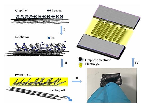
**Figure 11.** Preparation process of a micro-supercapacitor. (I) Electrochemical exfoliation of graphite foil. (II) Coating the graphene/graphite foil with gel electrolyte (PVA/H3PO4). (III) Peeling off flexible graphene paper-like electrode. (IV) Building of interdigitated micro-supercapacitor devices using the paper-like electrode. Reprinted with permission from ref. [110].
