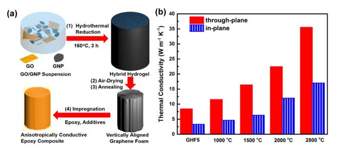
**Figure 6.** (a) Representative diagram of a conductive epoxy composite production enriched with vertically oriented RGO/GNP hybrid foam. (b) Thermal conductivity variation in the in-plane direction (red column) and in the transverse direction (blue column) of the epoxy composite incorporating the RGO/GNP hybrid foam aligned vertically at different temperatures. Adopted with permission from ref. [62].
