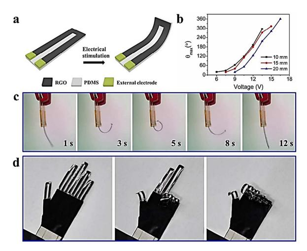
**Figure 10.** Fabrication of soft actuator with printed RGO electrodes. (**a**) RGO/PDMS bilayer actuator under electrical stimulation. (**b**) The maximum bending angle of the actuators as a function of the driving voltage. (**c**) Digital images of the actuator at various bending angles, with reversible shape change of the actuator. (**d**) The final look of a hand-shaped actuator with independent fingers controlled by various gestures. Reprinted with permission from ref. [105].
