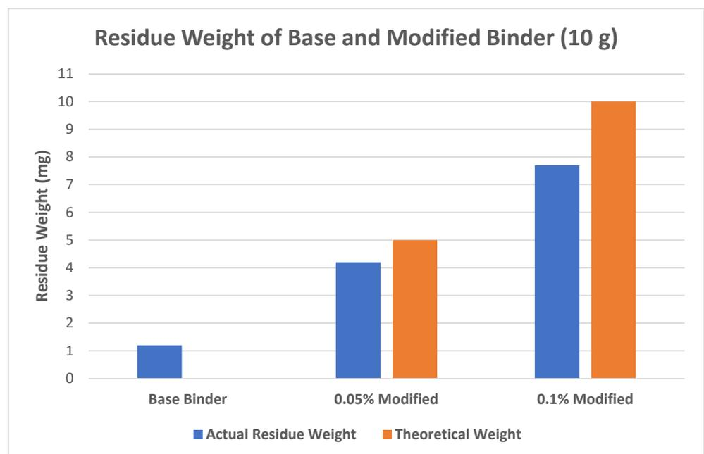
**Figure 11.** Residue weight of 10 g base binders and Zychotherm-modified binders.
