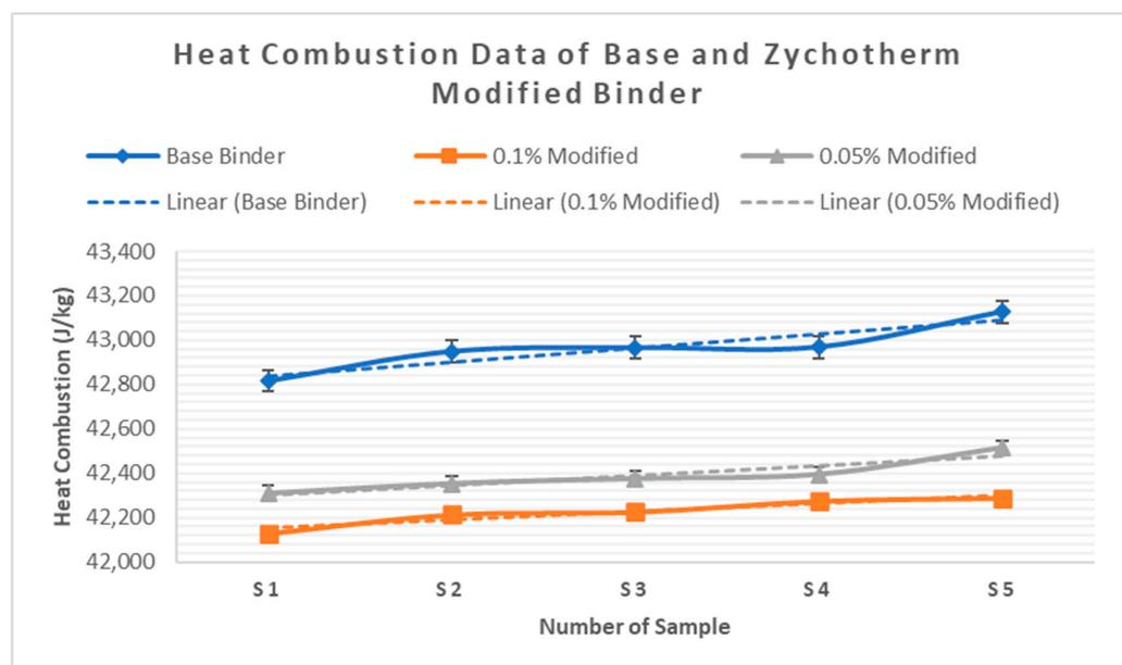
Figure 5. Heat combustion result of base binder and Zychotherm-modified binder (five repetitions for each sample) (reproduced).
