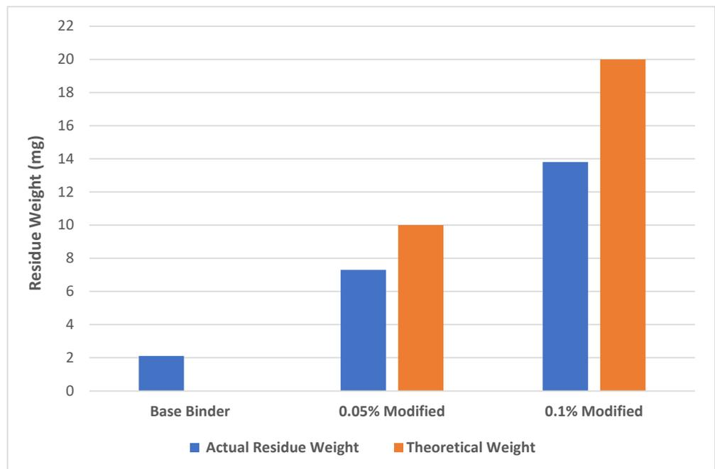
**Figure 10.** Residue weight of 20 g base binders and Zychotherm-modified binders.
