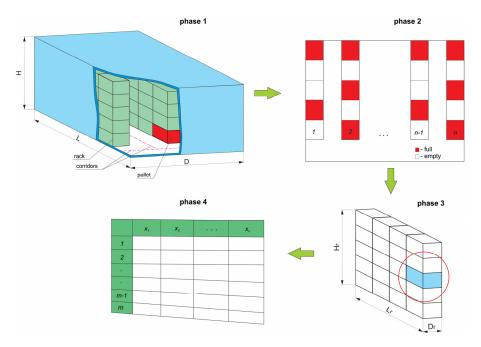
**Figure 2.** Schematic representation of the formation of a three-dimensional warehouse model and the procedure for obtaining the relevant parameters.
