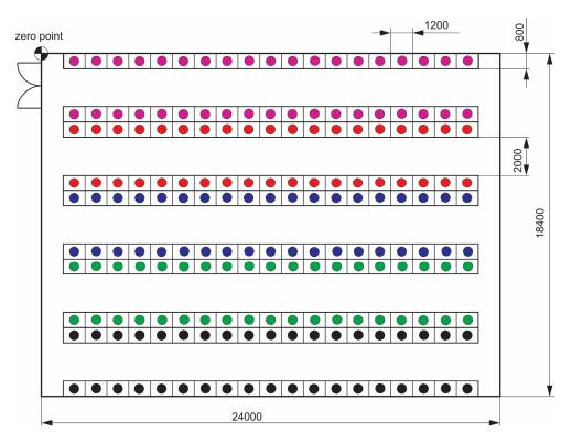
**Figure 4.** Layout of a high-bay warehouse with associated dimensions and materials (• wood, • cardboard, • chipboard, • PVC, and • rubber).
