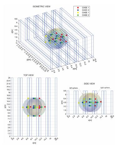
**Figure 5.** Graphic representation of the fire risk zones in the warehouse with isometric view, top view, and side view.
