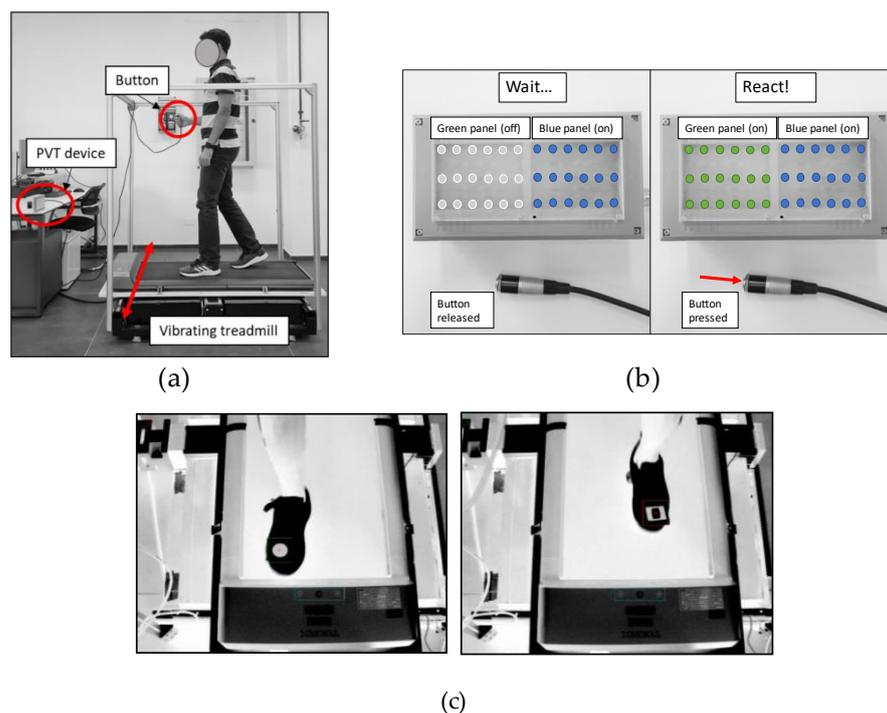
**Figure 1.** (a) Pictorial view of the setup: the vibrating platform and the PVT device; (b) PVT device: the subject waits a random amount of time (2–9 s) for the green LED to light up and then presses the button as quickly as possible to record the reaction time; (c) The patches on the feet to measure step width: a round shape on the right, and a square shape on the left.
