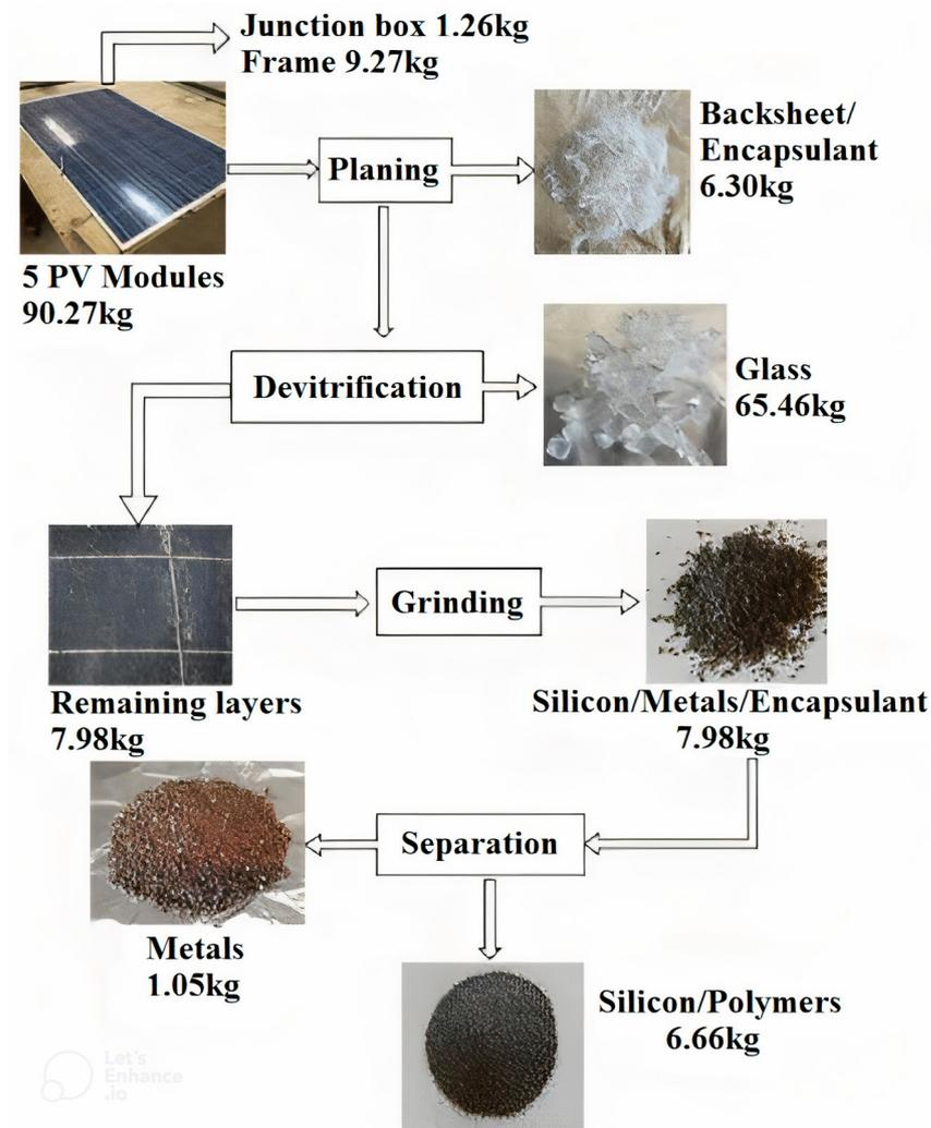
Figure 9. Management of photovoltaic (PV) solar panels that have reached their end of life [22].
