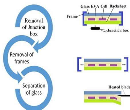
**Figure 7.** Delamination process by the hot-knife technique.
