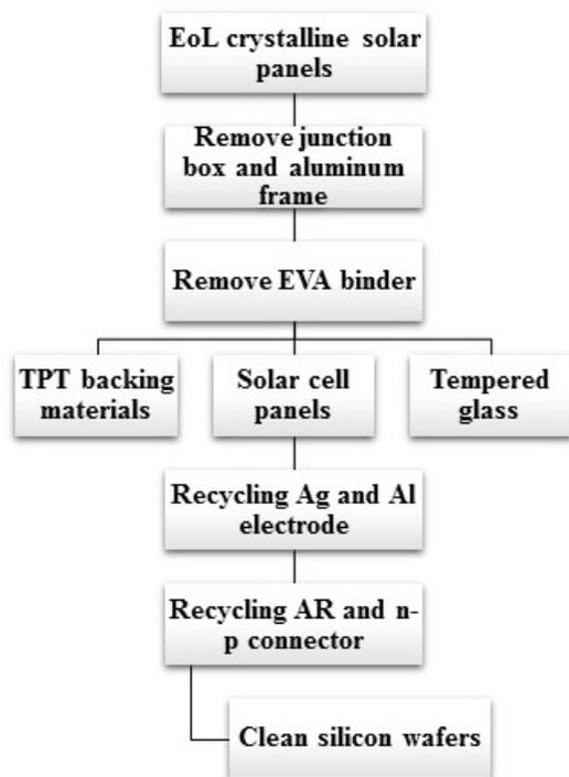
Figure 13. Recycling procedure for EOL solar panel [10].
