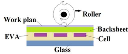
Figure 8. A side view of the surface delamination, grinding, and densimetric recycling technique.
