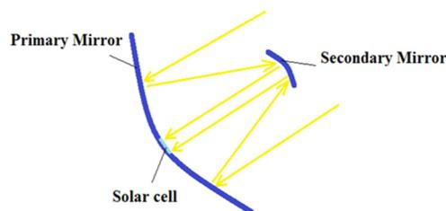
**Figure 3.** CPV structure.
