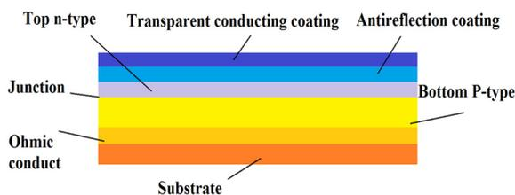
**Figure 4.** Structure of thin-film solar panels.
