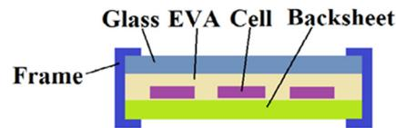
**Figure 2.** Structure of crystalline silicon solar panels.
