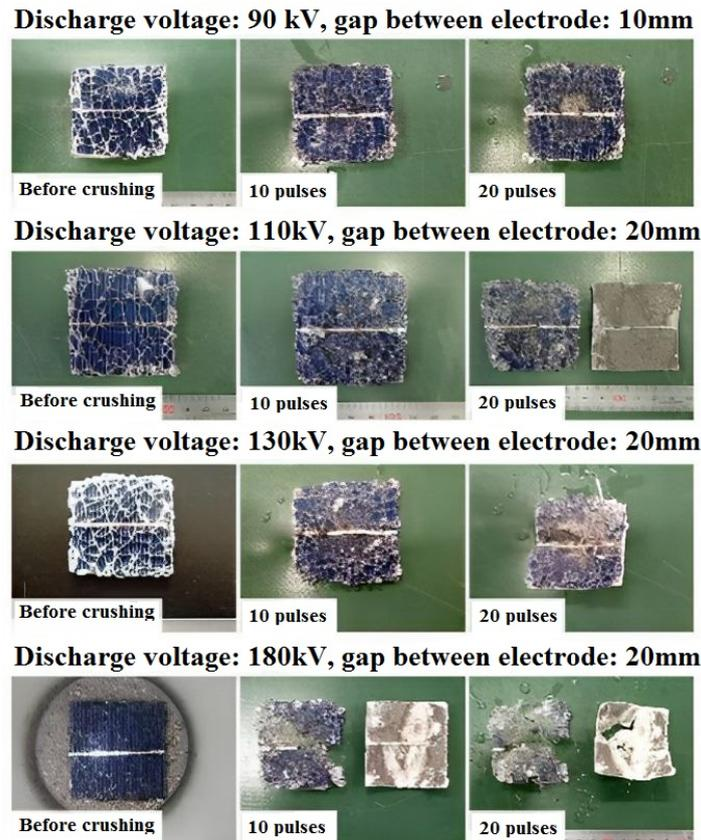
**Figure 11.** The products derived from the initial stage of high-voltage pulse crushing are subject to diverse conditions [26].
