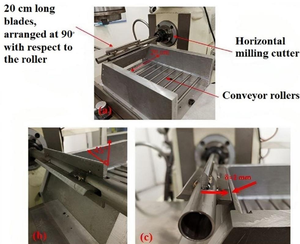
**Figure 10.** Specifications of the devitrifying machine. (a) A horizontal cutter and conveyor rollers. (b) Blade profile set at 45 degrees. (c) Distance between the roller blades and the inclined stator is 2 mm [22].
