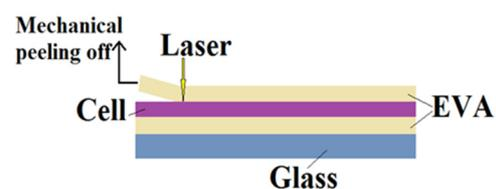
**Figure 12.** Delamination via laser irradiation.
