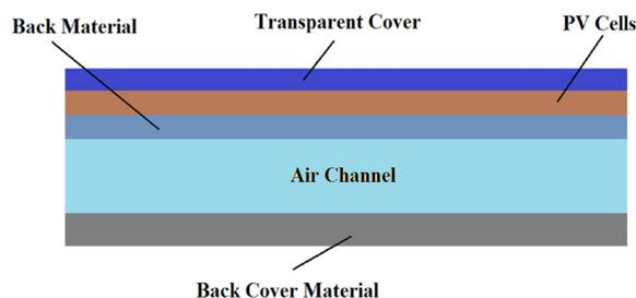
**Figure 5.** Air-based hybrid solar panel structure.
