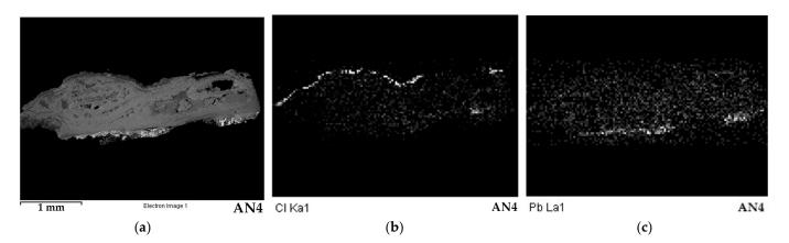
**Figure 7.** Other elements identified through SEM/EDS analysis on AN4: (**a**) backscattered electron image; (**b**) Cl; (**c**) Pb.
