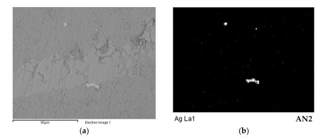
Figure 9. Silver identified through SEM/EDS analysis on AN2: (a) backscattered electron image; (b) Ag.
