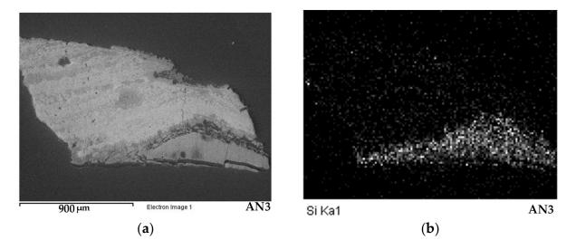
Figure 8. Silicon identified through SEM/EDS analysis on AN3: (a) backscattered electron image; (b) Si.
