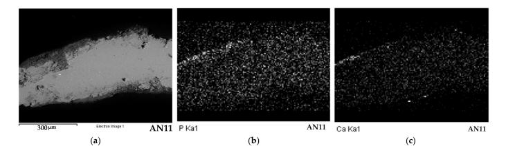
**Figure 6.** Other elements identified through SEM/EDS analysis on AN11: (**a**) backscattered electron image; (**b**) P; (**c**) Ca.
