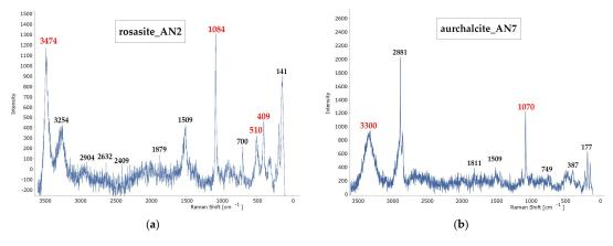
**Figure 10.** Copper and zinc hydroxide carbonates identified through Raman analysis; labels of characteristic peaks of corrosion products are highlighted in red: (a) rosasite on AN2; (b) aurichalcite on AN7.
