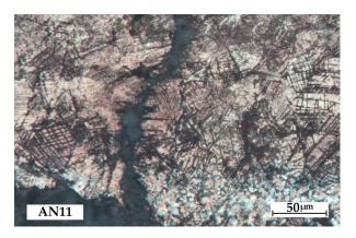
Figure 4. AN11 (brass fragment): slip bands highlighted by chemical etching with FeCl<sub>3</sub>/HCl.
