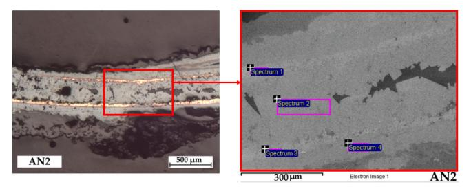
**Figure 3.** SEM-EDS image of the cross-section of AN2 (brass fragments). Pink boxes, corresponding to the spectra 1–5 showed in Table 3, correspond to analysed areas of AN2 cross-section.
