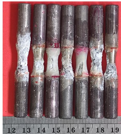
**Figure 4.** Samples after the corrosion test, with and without corrosion products.
