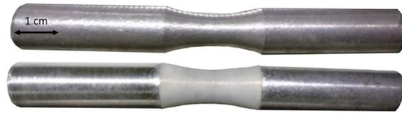
**Figure 1.** The fatigue standard sample with and without coating before corrosion.
