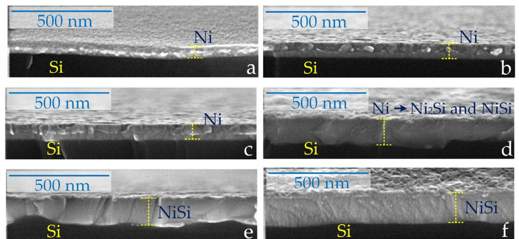
**Figure 1.** SEM images of the cross section of films on silicon: (a) before rapid thermal treatment; (b) after rapid thermal treatment at 200 °C; (c) after rapid thermal treatment at 250 °C; (d) after rapid thermal treatment at 300 °C; (e) after rapid thermal treatment at 350 °C; (f) after rapid thermal treatment at 500 °C.
