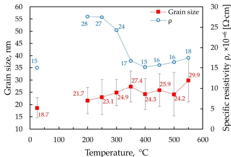
**Figure 6.** The specific resistivity and grain size of films before and after rapid thermal treatment.
