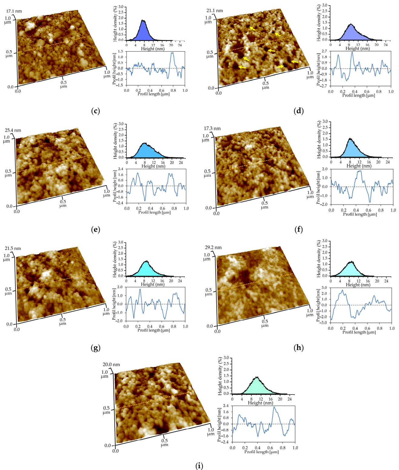
**Figure 3.** Microstructure with height distribution and profiles (in a field of  $1 \times 1 \mu\text{m}^2$ ) of the film surface before (a) and after (b–i) RTT: (a) 20 °C; (b) 200 °C; (c) 250 °C; (d) 300 °C; (e) 350 °C; (f) 400 °C; (g) 450 °C; (h) 500 °C; (i) 550 °C.
