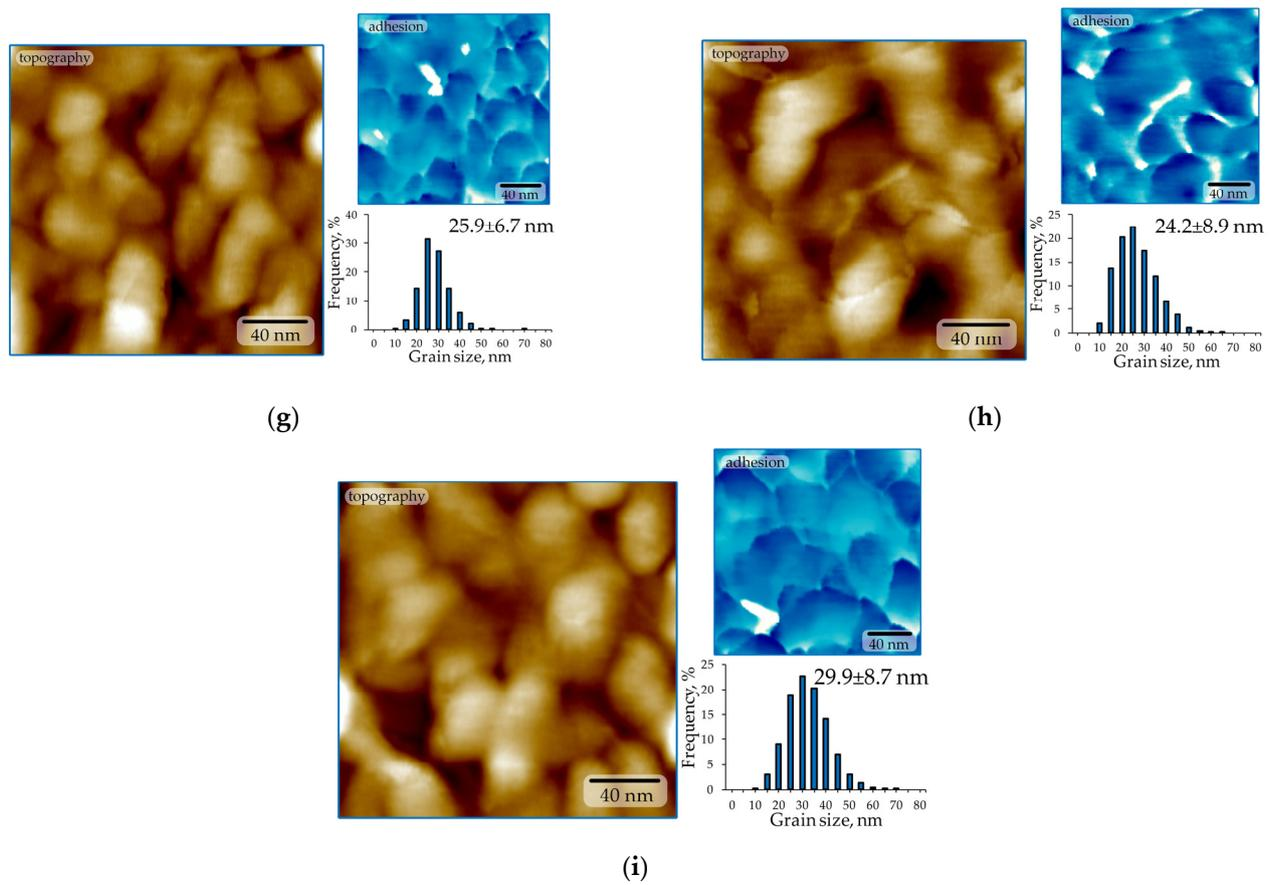
**Figure 4.** Microstructure of the film's surface with adhesive contrast (field  $200 \times 200 \text{ nm}^2$ ) and histograms of grain size distribution before (a) and after RTT (b–i) (a) 20 °C; (b) 200 °C; (c) 250 °C; (d) 300 °C; (e) 350 °C; (f) 400 °C; (g) 450 °C; (h) 500 °C; (i) 550 °C.
