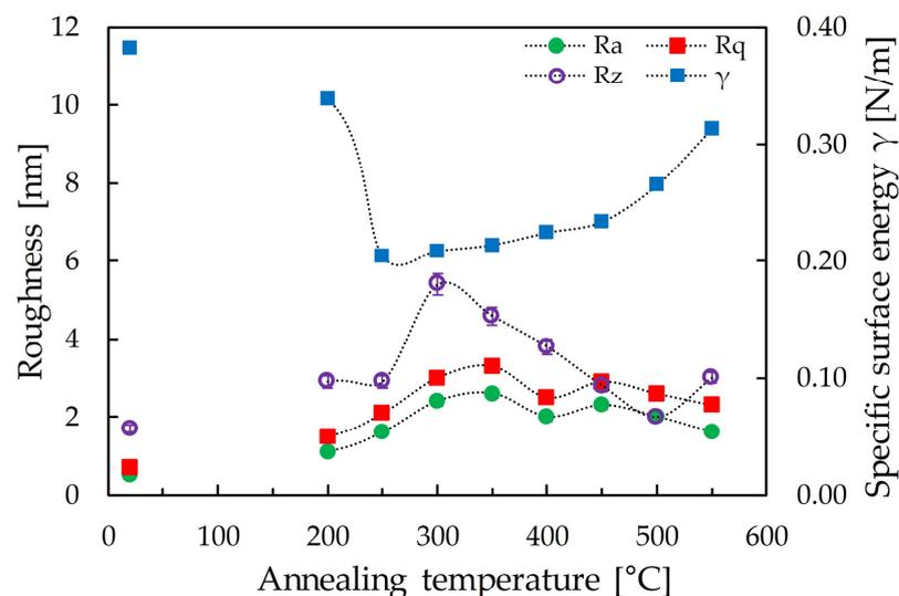
**Figure 5.** Film surface roughness and specific surface energy (field  $1 \times 1 \mu\text{m}^2$ ) before and after rapid thermal treatment.
