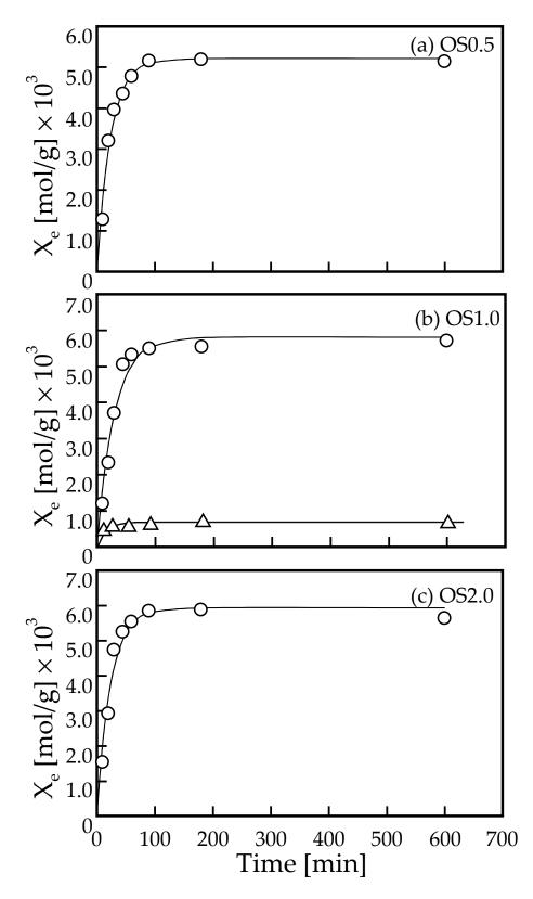
**Figure 4.** Time course of the amount adsorbed of Pb onto (**a**) OS0.5, (**b**) OS1.0, and (**c**) OS2.0 adsorbents. The solid curves in the figures were the calculated values using adsorption kinetic parameters determined by fitting of the data to Langmuir adsorption rate equation expressed by Equation (3). The triangle symbol corresponds to the amount adsorbed of Pb onto a non-modified shell particles (control).
