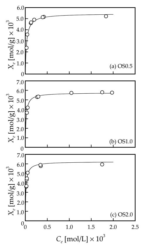
**Figure 5.** The adsorption equilibrium relationships of (**a**) OS0.5, (**b**) OS1.0, and (**c**) OS2.0 adsorbents and Pb, respectively. The solid curves in the figures were the calculated values using adsorption parameters determined by fitting of the data to Langmuir adsorption isotherm expressed by Equation (4).
