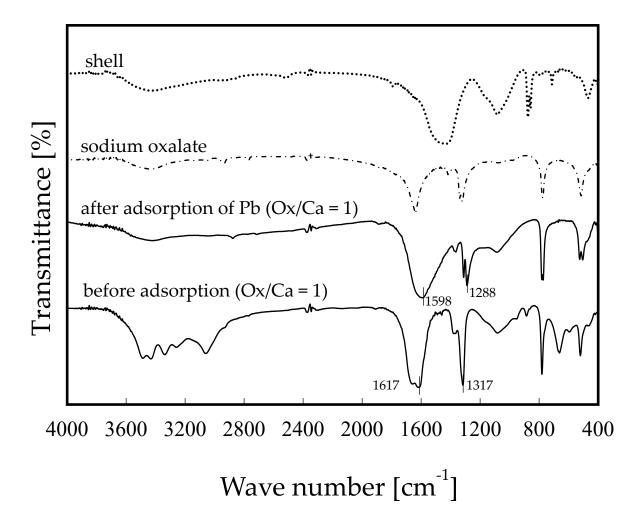
Figure 6. Comparison of FT-IR spectra of before and after the adsorption of lead ions for OS1.0.
