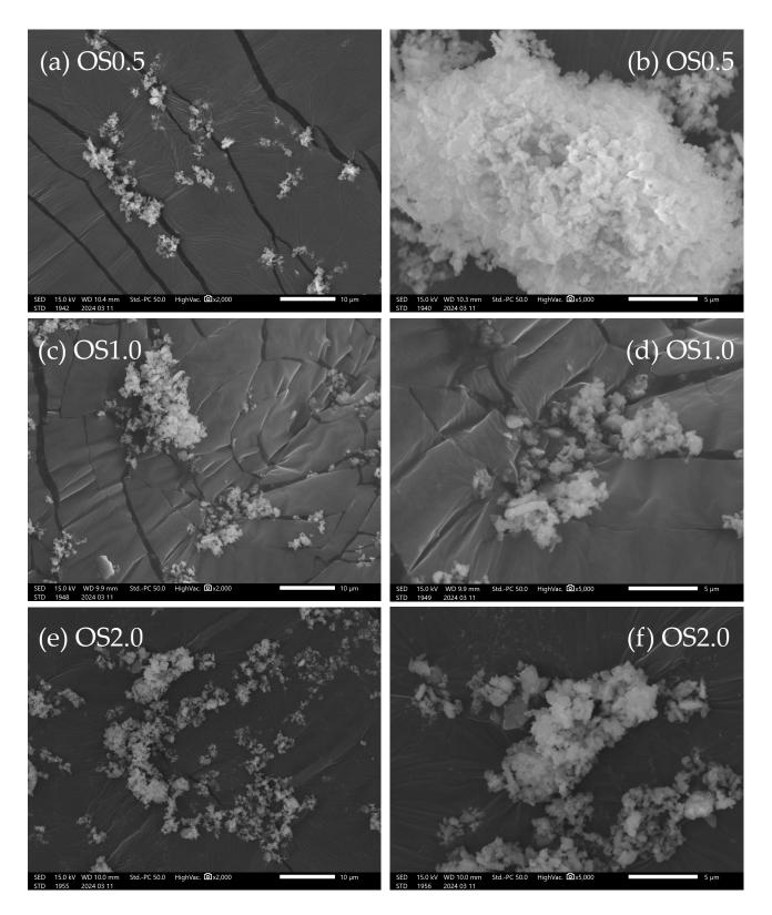
Figure 1. SEM images of the OS adsorbents: OS0.5 (a,b), OS1.0 (c,d), and OS2.0 (e,f).
