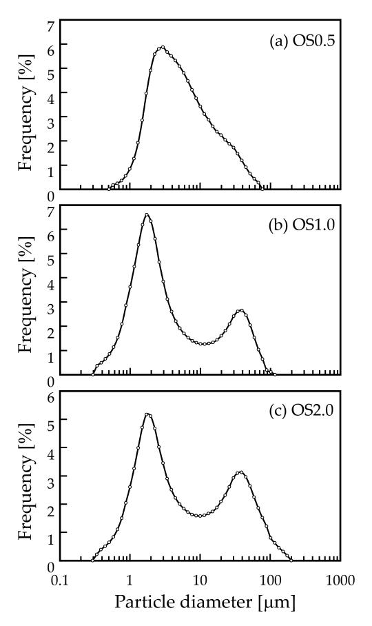
Figure 2. Particle size distribution of (a) OS0.5, (b) OS1.0, and (c) OS2.0 adsorbents.
