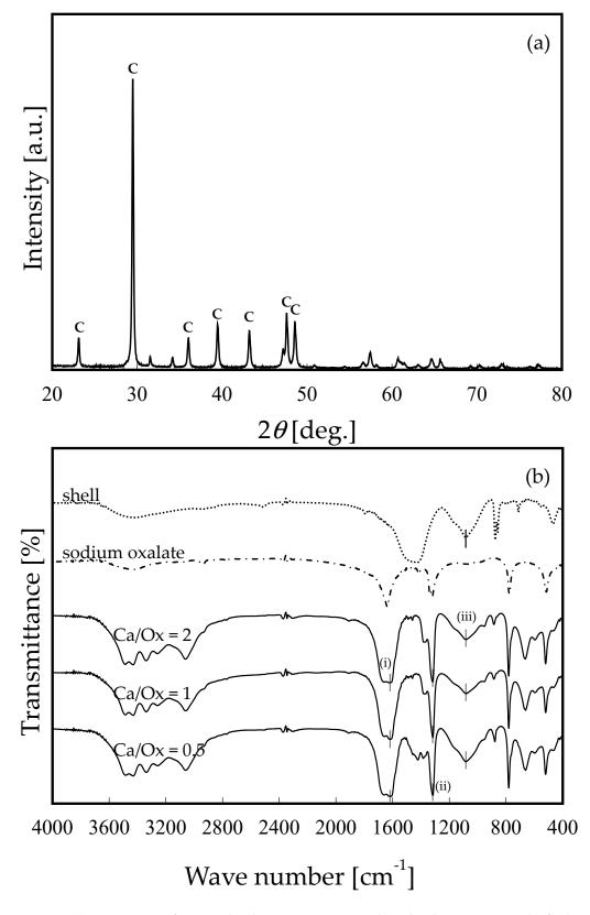
**Figure 3.** (a) XRD pattern of OS1.0. The character C corresponds to the characteristic peak of calcite (JCPDF: 01-078-4614, 04-008-0788). (b) FT-IR spectra of the prepared adsorbent particles with varying molar ratio before adsorption experiments.
