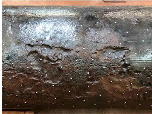
**Figure 6.** Localized corrosion predominantly on the undersides of cast iron pipe (900 mm dia., 100+-year-old, 1.2 m depth) in sandy loam soil.
