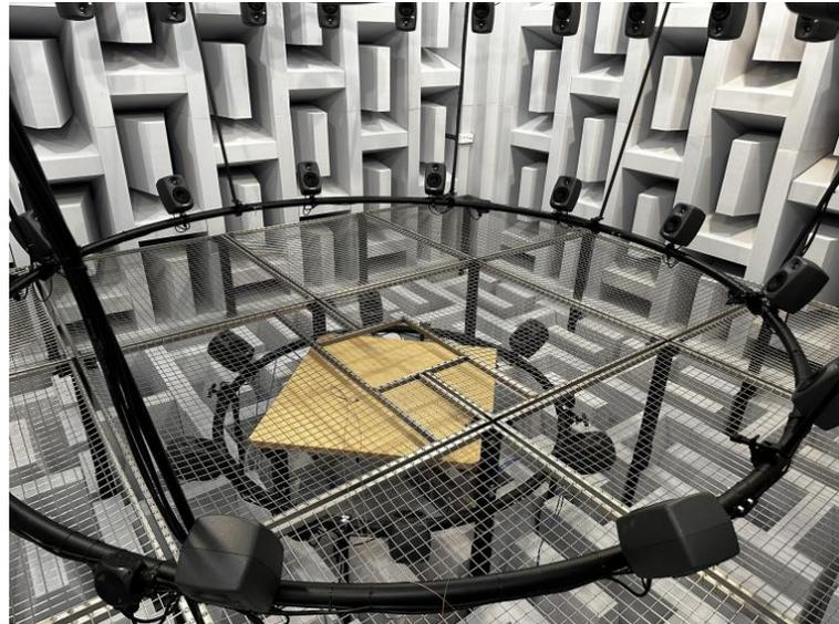
**Figure 6.** Photo of the vibration exposure device (VED) installed in the central position of the ambisonics reproduction system.
