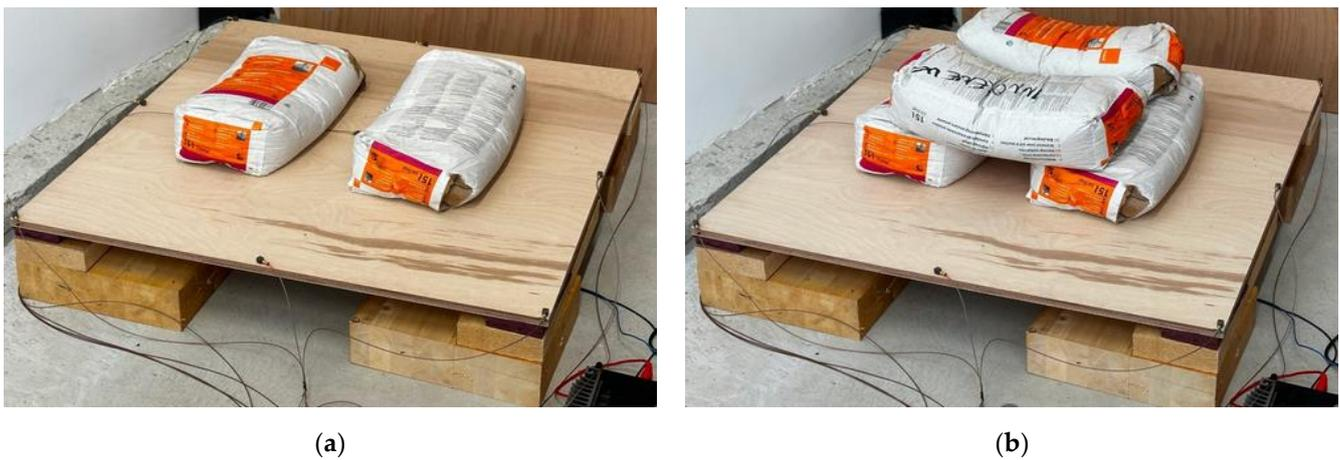
**Figure 7.** Loading of the platform (not yet installed in the anechoic chamber) during the preliminary frequency response measurements at a load of 45 kg (a) and 90 kg (b).
