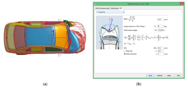
**Figure 14.** (a) Deformation of Toyota Yaris after the collision with the pole/tree object; (b) "Crash 3—EBS Calculation 12.0" calculation window.
