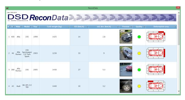
**Figure 7.** EES catalog with examples of various car deformations for setting the EES parameter:
