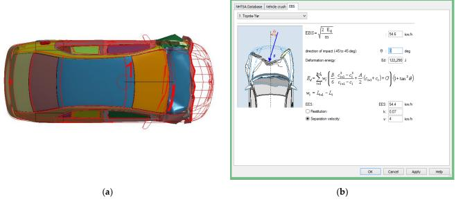
**Figure 15.** (a) Deformation of Toyota Yaris after the collision with the non-deformable wall; (b) "Crash 3—EBS Calculation 12.0" calculation window.
