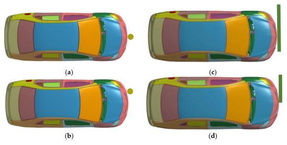
**Figure 8.** Visual view of the Toyota Yaris before collision: (a) impact velocity—50 km/h, object—200 mm pole, object position—center; (b) impact velocity—50 km/h, object—200 mm pole, object position—25% offset; (c) impact velocity—50 km/h, object—wall, object position—100% overlap; (d) impact velocity—50 km/h, object—wall, object position—50% overlap.
