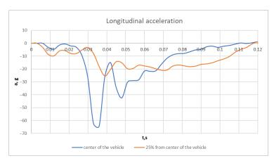
**Figure 12.** Longitudinal acceleration upon impact of the car with a solid object having a diameter of 200 mm.
