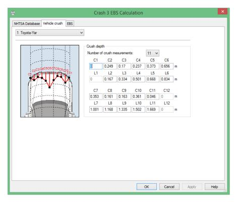
Figure 5. Dividing the width of the damage (deformation) of the test vehicle into segments.
