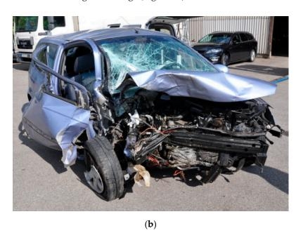
**Figure 16.** Frontal deformation image of a Hyundai Getz of the same class in the EES catalog: (a) top view; (b) front view.
