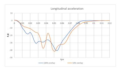
Figure 13. Longitudinal acceleration upon impact of the car with the non-deformable wall.
