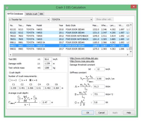
Figure 4. Calculation of A, B, and G coefficients in "Crash 3—EBS Calculation 12.0".
