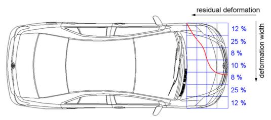
Figure 3. Marking the depth of residual deformation.
