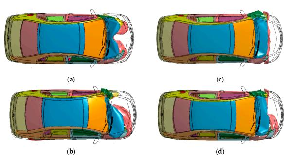
**Figure 9.** Visual view of the Toyota Yaris after collision: (a) impact velocity—50 km/h, object—200 mm pole, object position—center; (b) impact velocity—50 km/h, object—200 mm pole, object position—25% offset; (c) impact velocity—50 km/h, object—wall, object position—100% overlap; (d) impact velocity—50 km/h, object—wall, object position—50% overlap.
