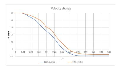
Figure 11. Velocity change upon impact of the car with the non-deformable wall.
