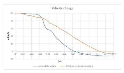
Figure 10. Velocity change upon impact of the car with the 200 mm diameter solid object.
