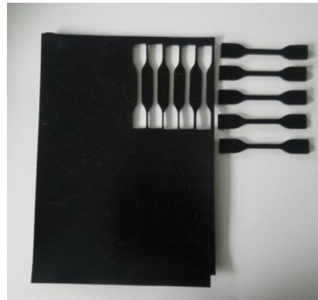
**Figure 3.** Image of the test specimens used for uniaxial tensile tests. The dimensions of the specimens correspond to those of standard specimens of type 5A in ISO 527 and type S2 in ISO 53504. The image corresponds to a PU-nanocomposite filled with 10 wt% Printex® 30.
