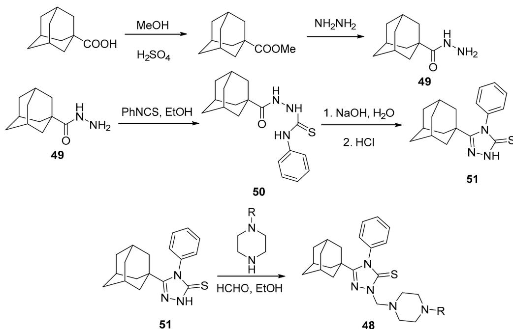
**Scheme 21.** Synthesis of 5-((3*r*,5*r*,7*r*)-adamantan-1-yl)-2-((4-alkylpiperazin-1-yl)methyl)-4-phenyl-2,4-dihydro-3*H*-1,2,4-triazole-3-thiones.
