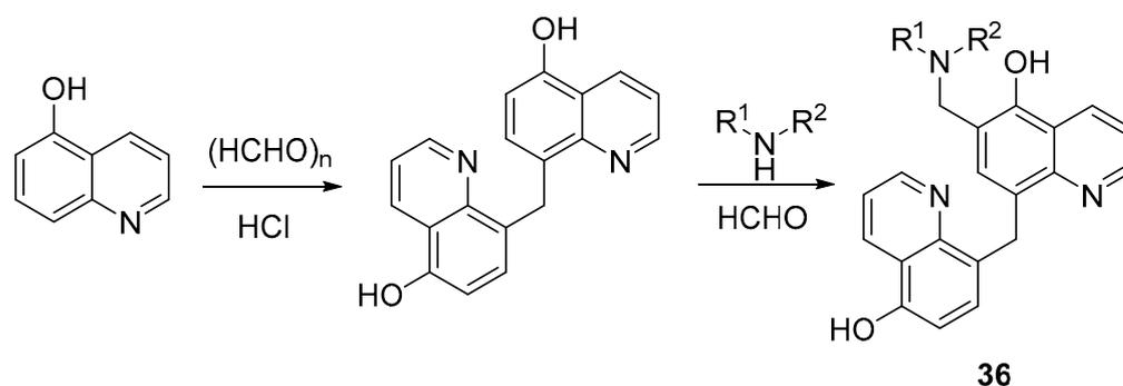
**Scheme 16.** Synthesis of Mannich bases derived from 8-hydroxyquinoline.
