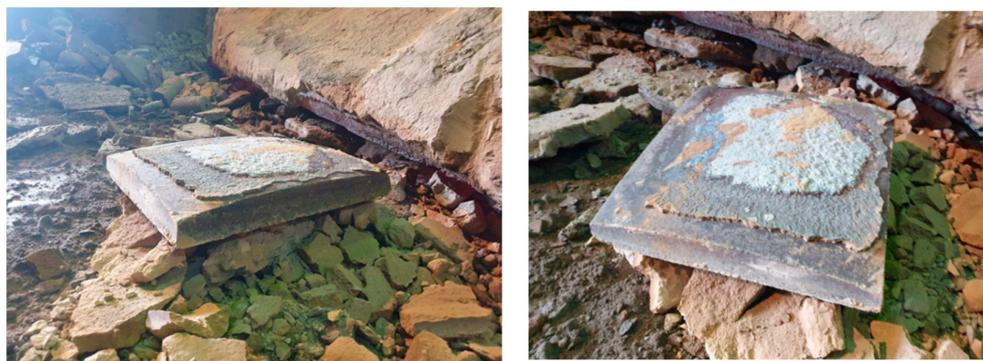
**Figure 3.** Post-casting examination of the spherical impact pad after 32 heats from diverse viewpoints.
