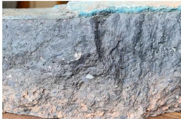
**Figure 4.** Fracture (observed in the laboratory) of the spherical impact pad in the area directly affected by the stream of cast steel after the casting of 32 heats (equivalent to 5760 tons of steel).
