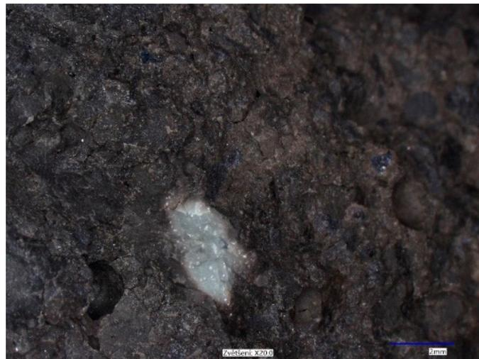
**Figure 5.** Material structure of the impact pad after use (magnification  $\times 20$ ).
