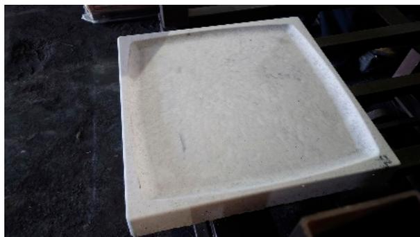
**Figure 2.** New developed special modification of “Spheric” impact pad for Delta tundish.
