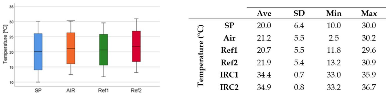
**Figure 3.** Bloxplot representation and descriptive statistics of the setpoint temperature (SP), the real air temperature (Air), the reflected temperatures measured with IR camera 1 (Ref1) and IR camera 2 (Ref2) and the point on the face with maximum temperatures measured with IR camera 1 (IRC1) and IR camera 2 (IRC2).
