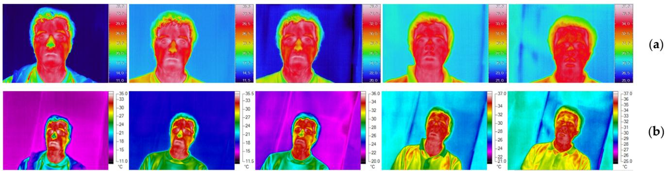
**Figure 4.** Thermal images taken during scenarios RH = 40% and T = 10 °C, RH = 40% and T = 16 °C, RH = 40% and T = 22 °C, RH = 40% and T = 26 °C and RH = 40% and T = 30 °C: (a) IR camera 1; (b) IR camera 2.
