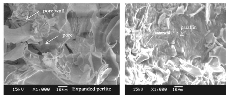
**Figure 1.** SEM images of expanded perlite (left) and paraffin-expanded perlite (right) [17].**Table 2.** Properties of typical commercial PCMs.
