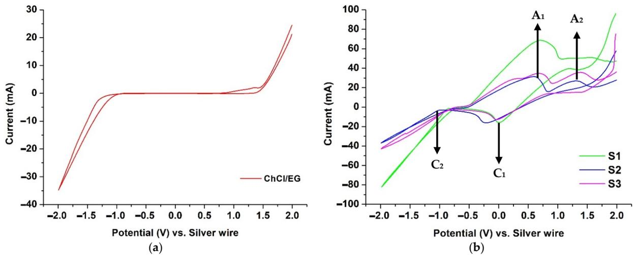
**Figure 1.** Cyclic voltammograms of (a) pure DES and (b) Fe and Fe–Mn bath electrolytes performed at 80 °C and 20 mV/s.
