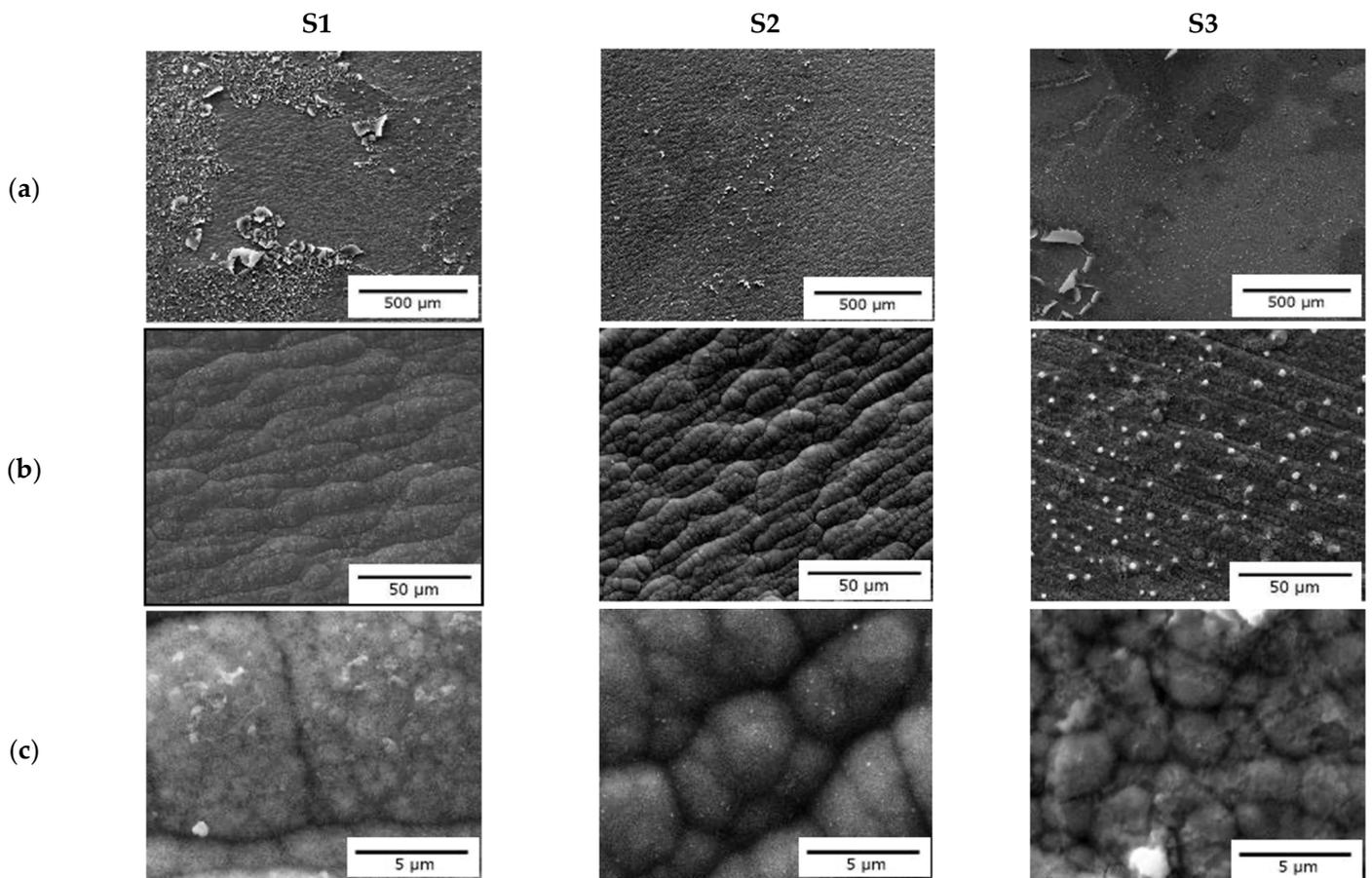
**Figure 3.** SEM images of the surface of deposits obtained for different concentrations of Fe–Mn and magnification of (a) 100 $\times$ , (b) 1000 $\times$ , and (c) 10,000 $\times$ .
