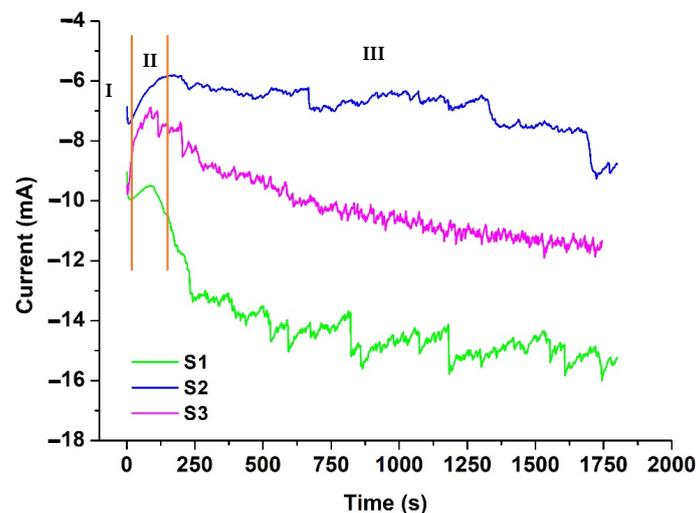
**Figure 2.** Experimental current density transients recorded during the electrodeposition onto the titanium substrate from the system ChCl/EG with Fe and Mn salt addition at 80 °C.
