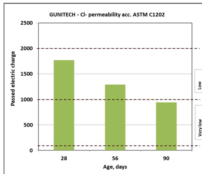
**Figure 1.** Chloride permeability according to ASTM C1202.
