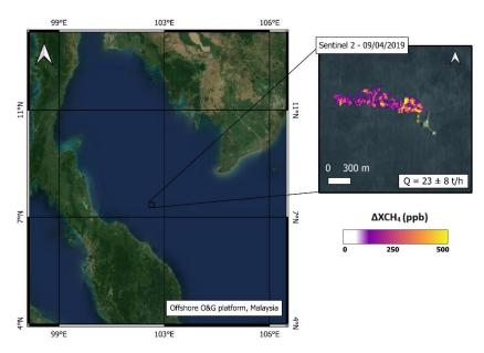
**Figure 1.** The right panel shows a methane emission from offshore O&G platform detected by Sentinel-2 satellite on 9 April 2019. The map on the left panel indicates the location of the platform in Malaysia.
