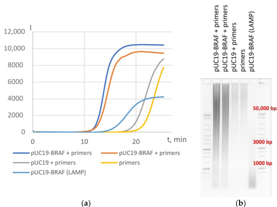
**Figure 6.** Amplification of the cloned BRAF gene using (a) real-time amplification and (b) agarose gel electrophoresis.
