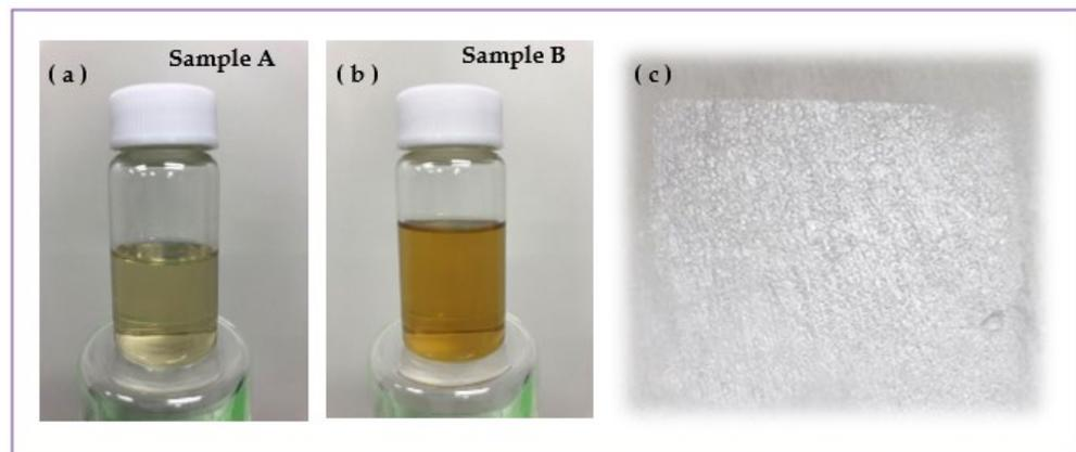
**Figure 3.** Colloids of Fe-containing NPs laser-generated in chloroform at 30 (a) and 120 mJ/pulse (b), and a PLLA nanosheet incorporated with such NPs (c) placed on polyester filter mat. The actual size of the NS in panel (c) is  $3 \text{ cm} \times 3 \text{ cm}$ .
