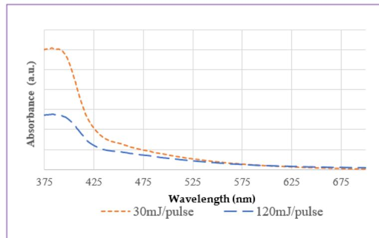
**Figure 7.** UV-visible spectra of Fe-based colloids prepared using ns-pulsed laser at 30 (orange) and 120 mJ/pulse (blue).
