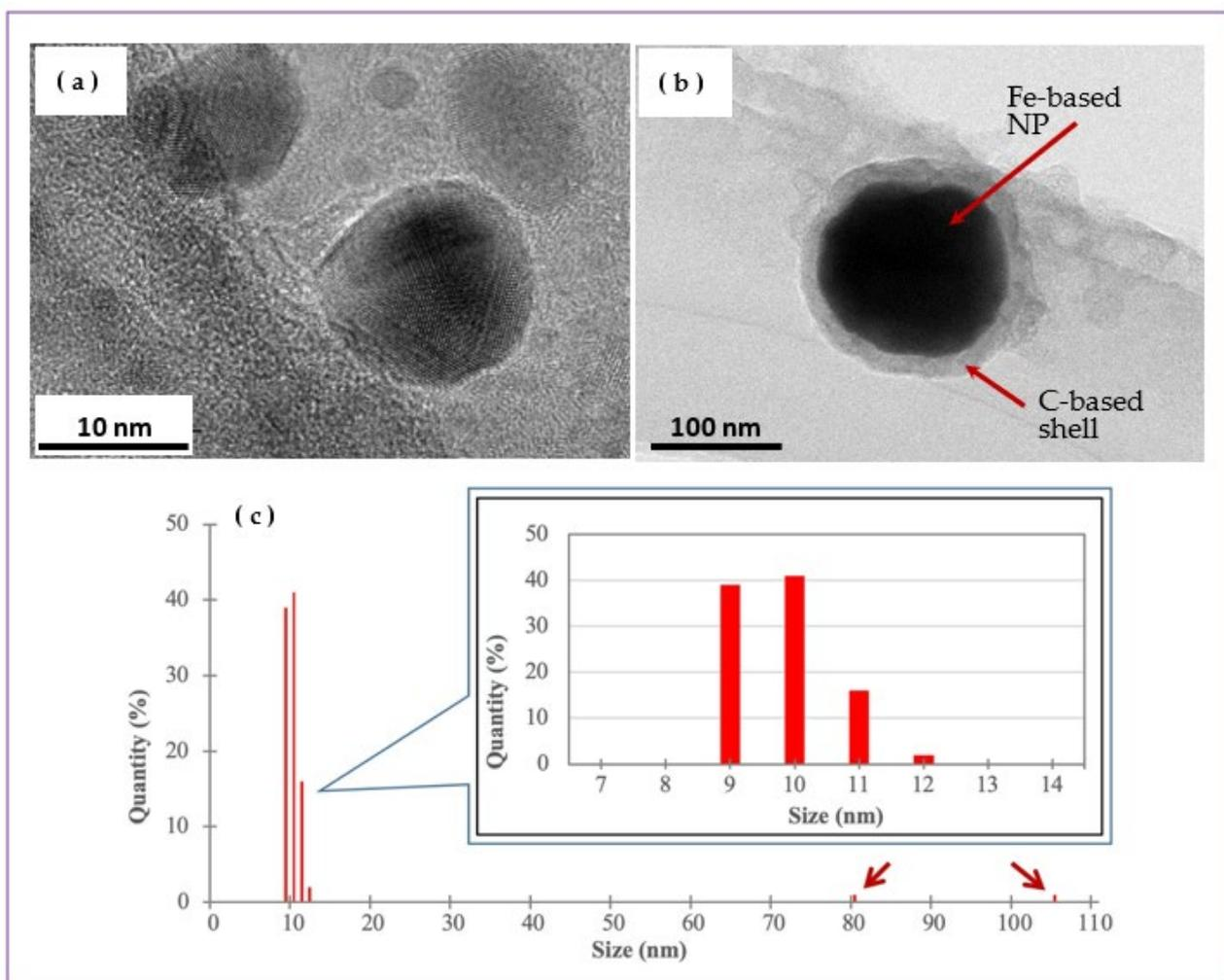
**Figure 5.** (a,b) TEM images of Fe-based NPs prepared at 30 mJ/pulse (Sample A): (a) small NPs and (b) larger NP with C-based shell. (c) Histogram of size distribution of Fe-containing NPs as measured by DLS. The two red arrows in panel (c) indicate bars for NPs with sizes ~81 and ~106 nm.
