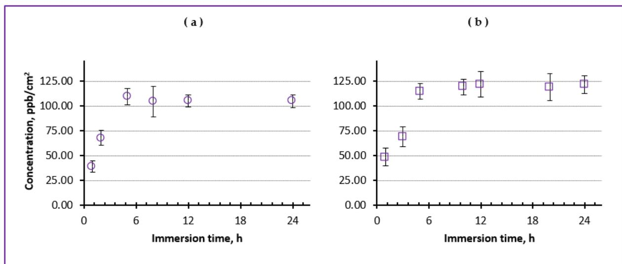
**Figure 10.** Concentration of Fe ions released by NSs incorporated with Fe-containing NPs laser-prepared at 30 (a) and 120 mJ/pulse (b). Both NSs were prepared using corresponding colloids with the same NP concentration (~0.3 mg/mL).
