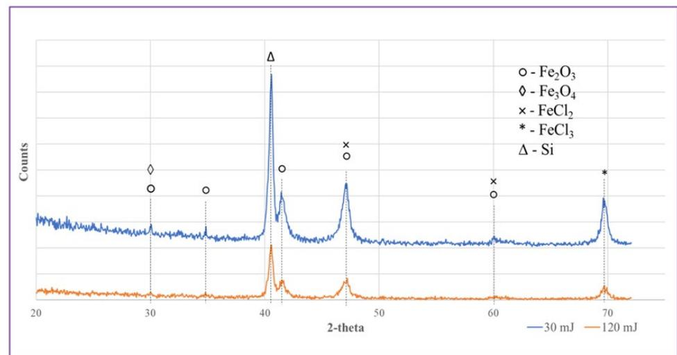
**Figure 9.** XRD patterns of Samples A (blue) and B (orange) prepared at 30 (blue) and 120 mJ/pulse (orange) and deposited on Si wafer.
