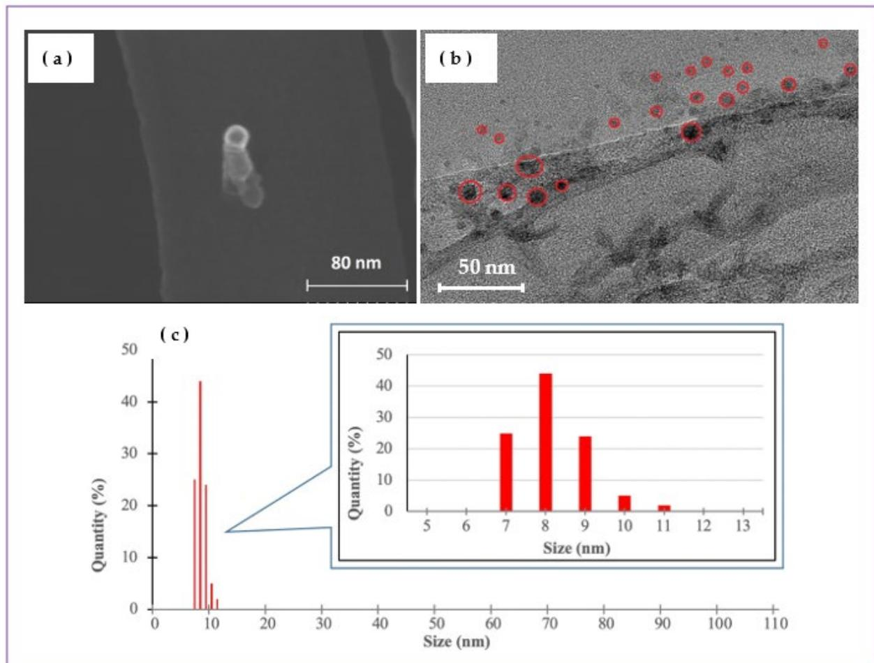
**Figure 6.** SEM (a) and TEM (b) images of Fe-based NPs prepared at 120 mJ/pulse (Sample B). (c) Histogram of size distribution of NPs in Sample B, as measured by DLS.
