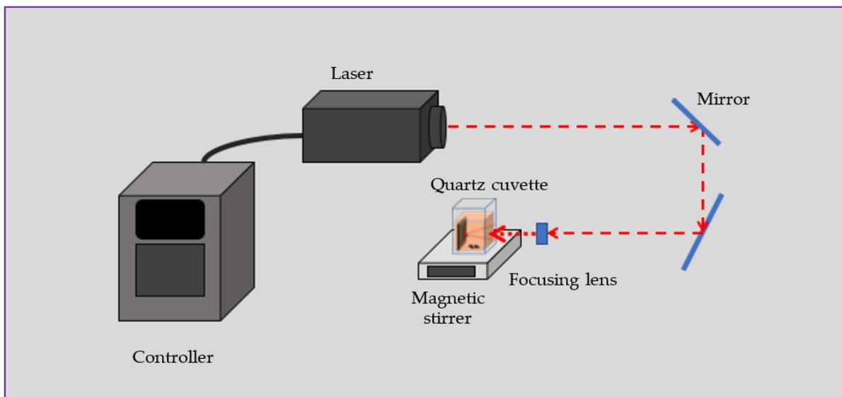
**Figure 1.** Setup with ns-pulsed laser used to produce nanoparticles via ablating iron plate in chloroform.
