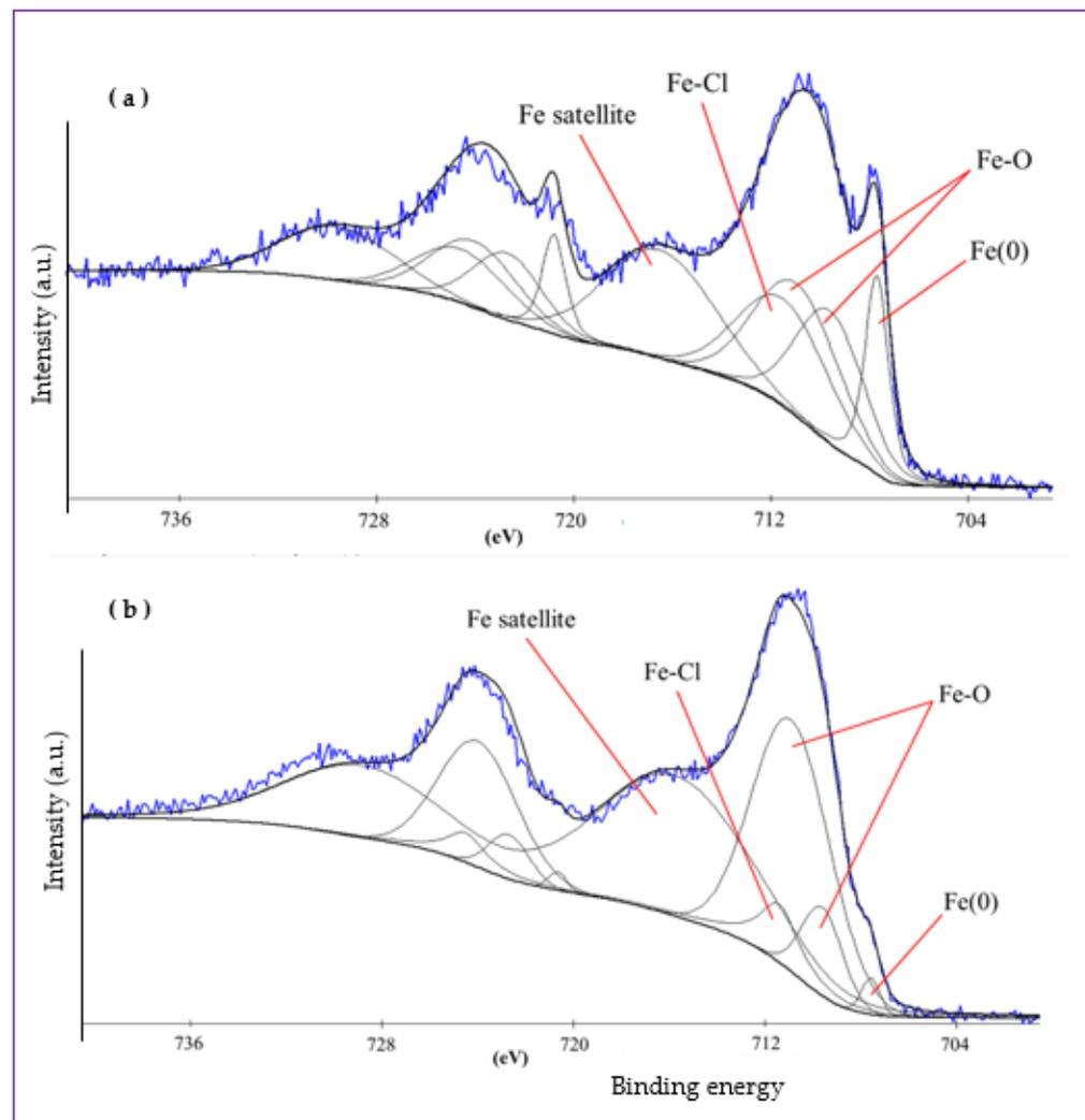
**Figure 8.** XPS Fe 2p spectra of Samples A (a) and B (b) prepared at 30 and 120 mJ/pulse, respectively. The blue curves present actual measured signal while the black curves are from curve-fitting.
