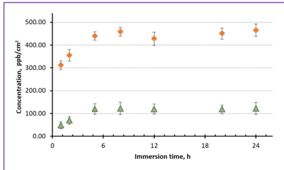
**Figure 11.** Concentration of Fe (triangles) and Zn (diamonds) ions released by NSs incorporated with two types of NPs. Sample B and commercial ZnO NPs (with sizes below 25 nm) were used as source of Fe and Zn ions, respectively.
