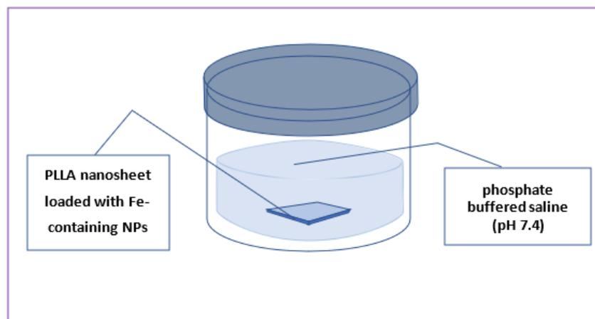
**Figure 4.** Experimental set-up used for ion-release test.
