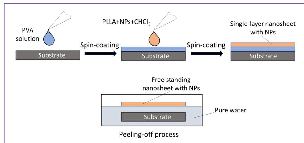
**Figure 2.** Fabrication of PLLA nanosheet incorporated with nanoparticles.
